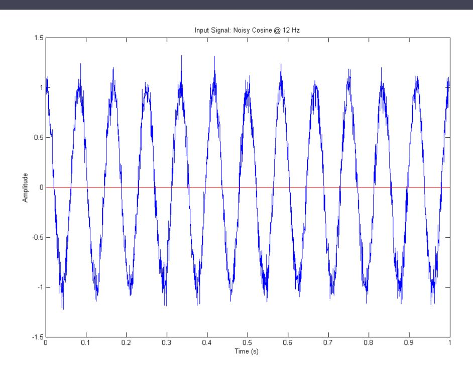
Since the DFT is invertible, it can be used for noise removal, by transforming a signal, using window functions to remove undesired components, and inverting the transform.
