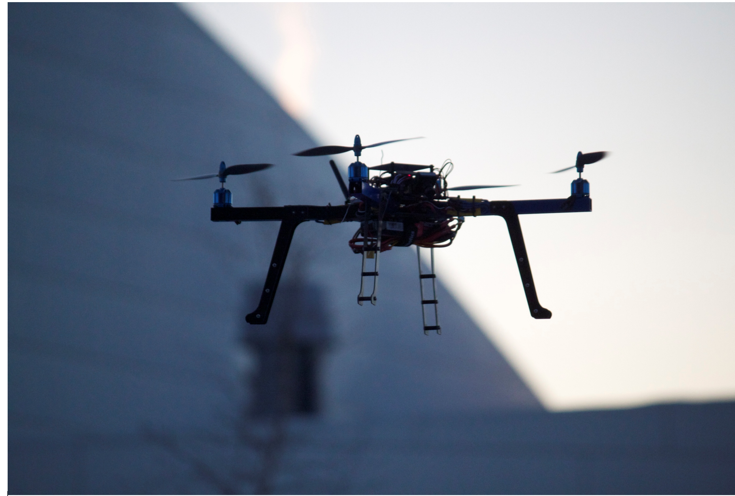
Fully assembled Quad-Rotor UAV flying with the APM 2.5 autopilot system. Calibration and tuning had to be done in order to achieve a stable flight. During the first flight, using the default flight control settings, the UAV was shaking violently and any control input was so greatly exaggerated that the UAV ended up crashing when it flipped over after being told to "Turn Left". Several more flights would be necessary to attain a stable flight as settings were adjusted and tested.
