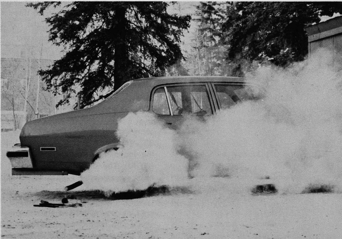
Fig. 10 1974 Nova with cooler-condenser bypassed. (-30°F ambient)
