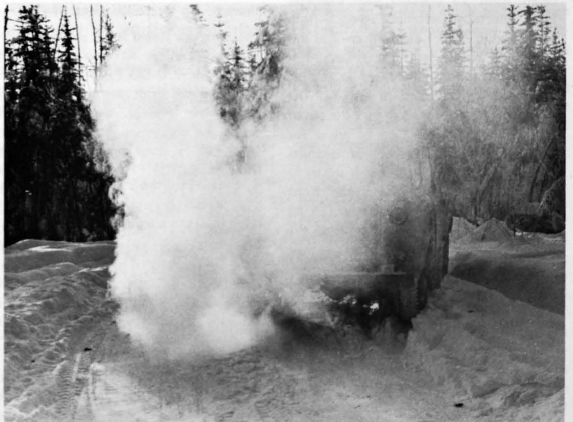
Fig. 7 1968 Scout exhaust without ice fog control.
