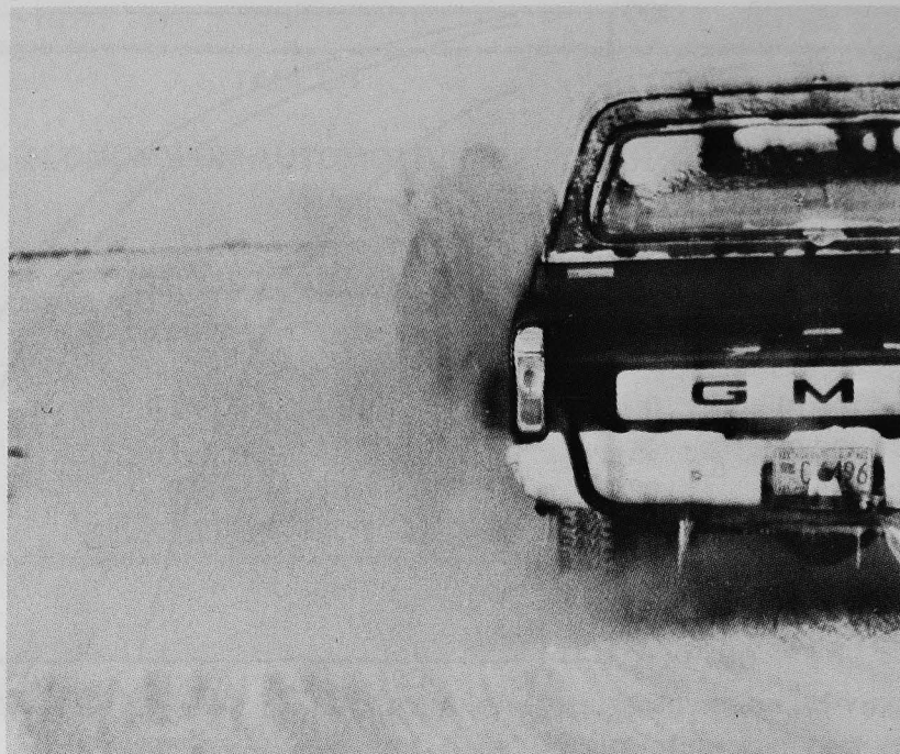
Fig. 4 Exhaust visibility without ice fog control device.
