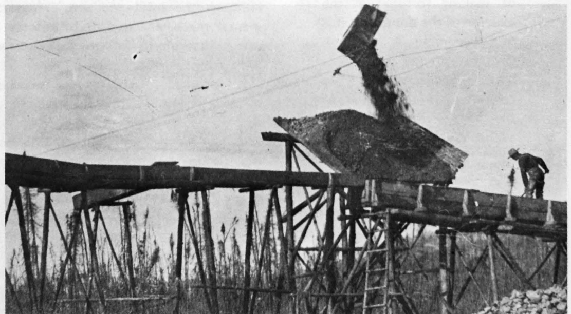
A bucket dumps gravel into an elevated sluice where a miner removes large rocks and prepares the pay dirt for sluicing. (Courtesy of Clara Rust Collection, Archives, University of Alaska, Fairbanks.)
