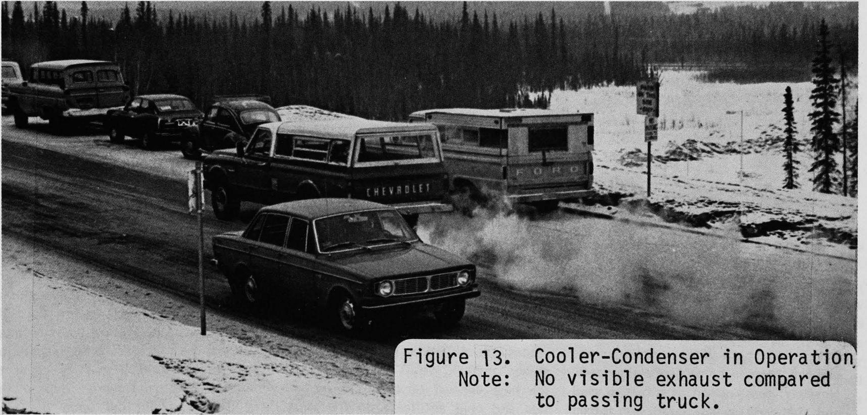
Fig. 13 Cooler-condenser in operation. Note: No visible exhaust compared to passing truck.
