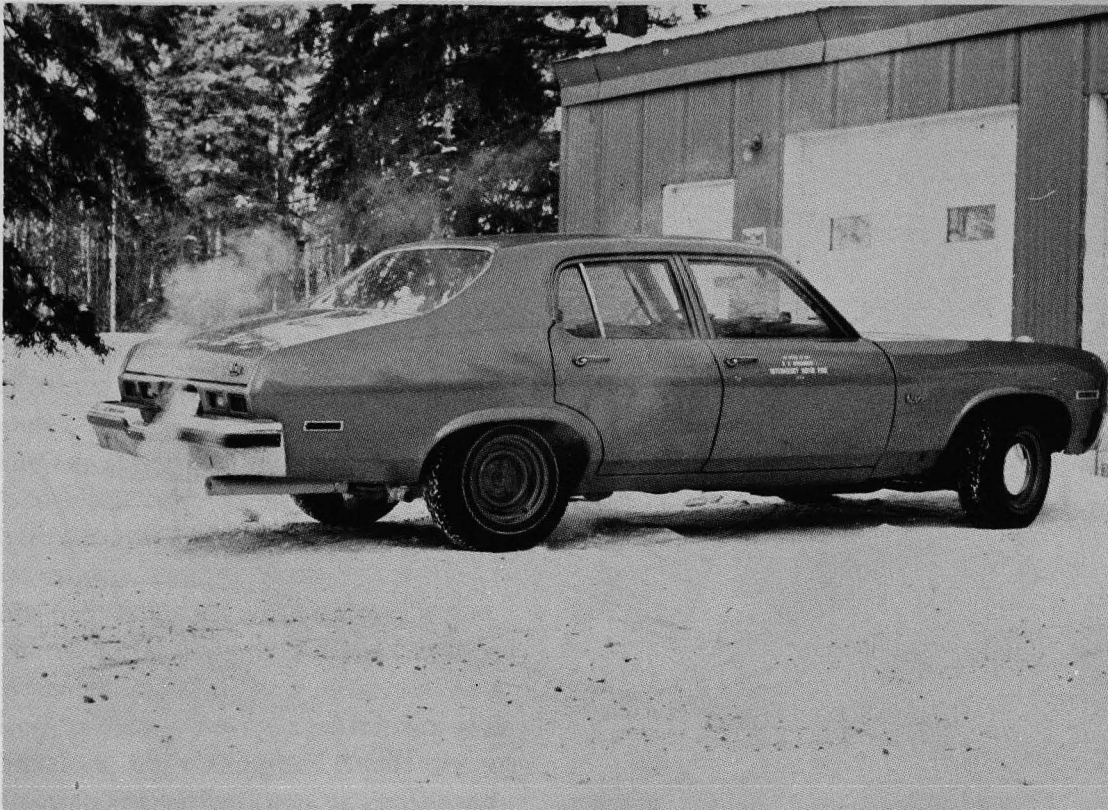
Fig. 9 1974 Nova with cooler-condenser outlet through rear coalescer. (-30°F ambient)
