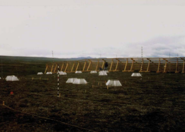
Figure 8. Snowfence experiment within the Toolik Lake Grid, summer view showing fence, snow-depth monitoring stakes, and small open-top greenhouses.
