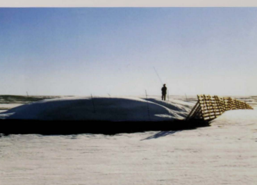
Figure 9. Winter view of snowfence experimental area showing the drift that forms behind the fence. Tall stakes are the same as striped stakes in Figure 8.
