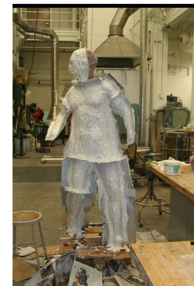
Brushing on the liquid plastic two part mother mold to ¼ inch minimum, two coats used
