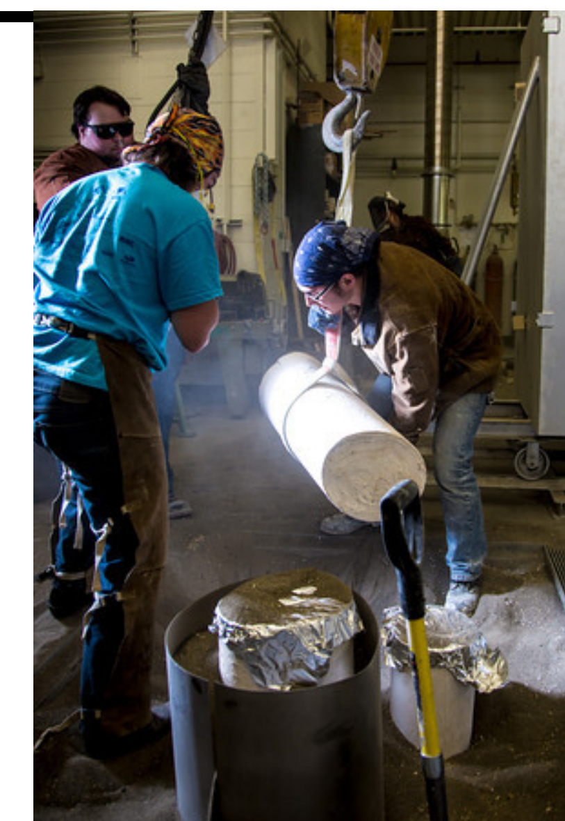
The molds have been are vacuumed out, aluminum foil is placed over the pour cup.
