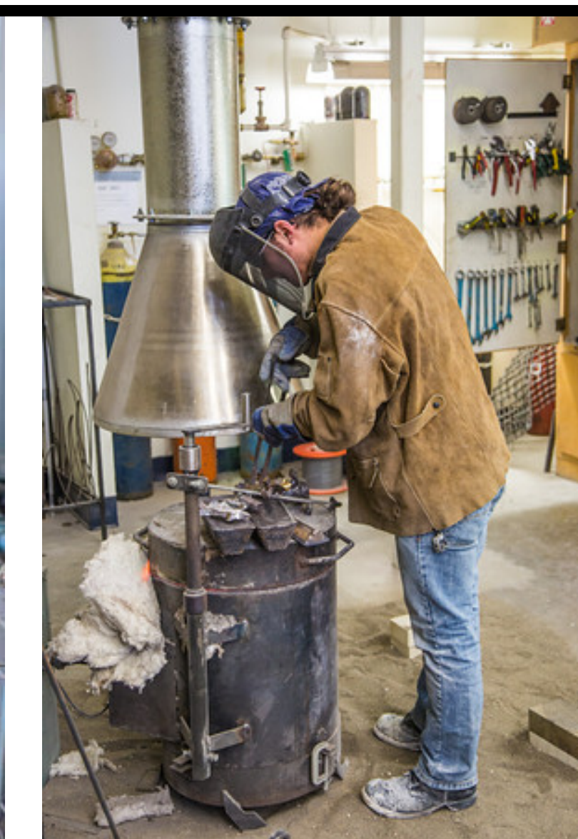
Preheating the metal to go into the furnace. Metal must be preheated before being added to the crucible (moisture touching molten metal can cause an explosion).
