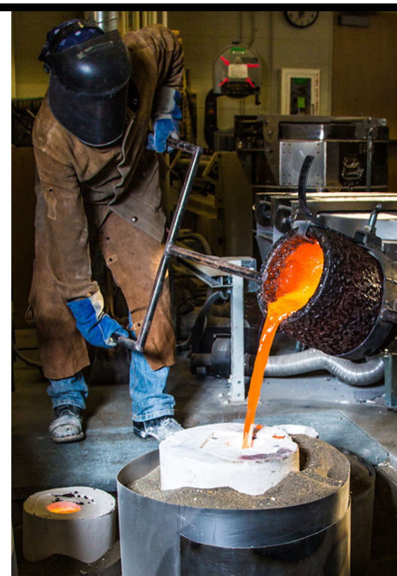
Pouring the molten bronze into the mold, bronze melts at about 1700 F and is poured between 1780 F and 1900 F.
