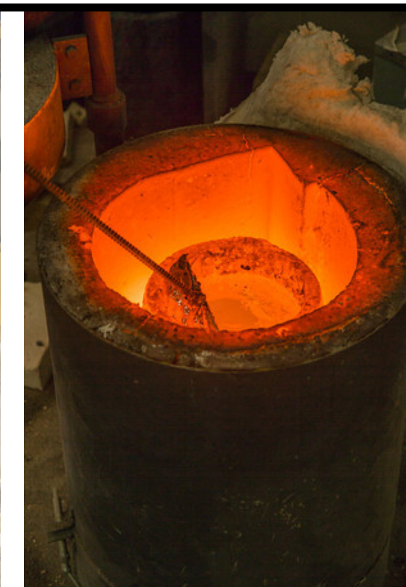
A preheated skimmer is used to remove the slag (impurities) that rise to the surface of the molten bronze.
