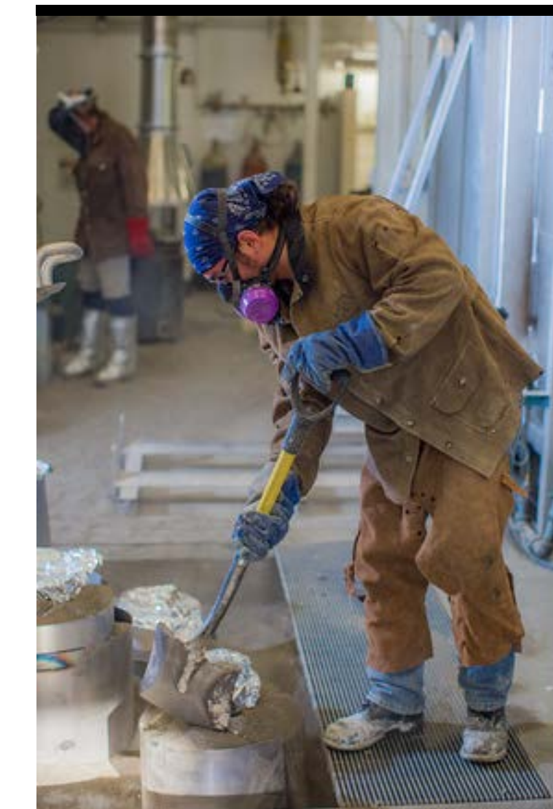
Placing steel rings around the molds and filling with sand for support.
