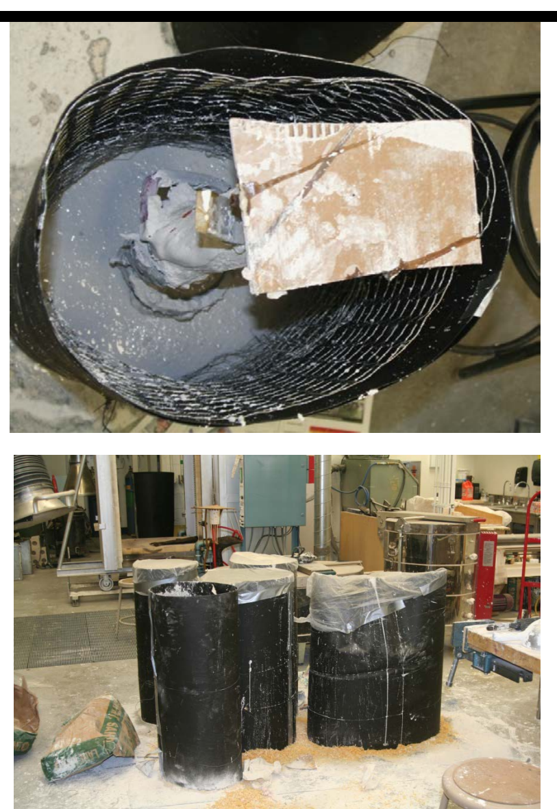
Plaster Silica Molds are poured ready to be loaded in the kiln for burn out firing for three days
