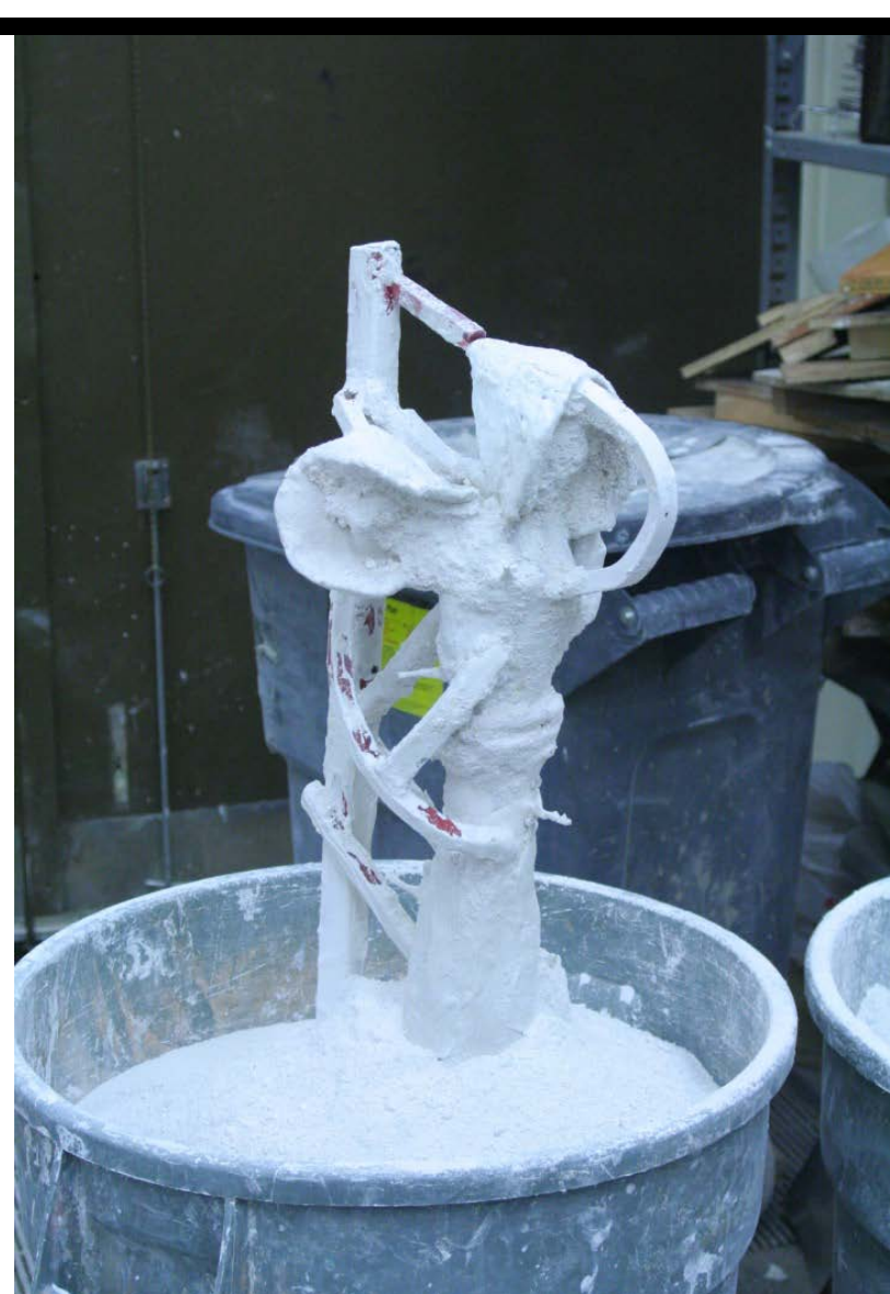
Applying silica plaster face coat over Shellac and alcohol mixture
