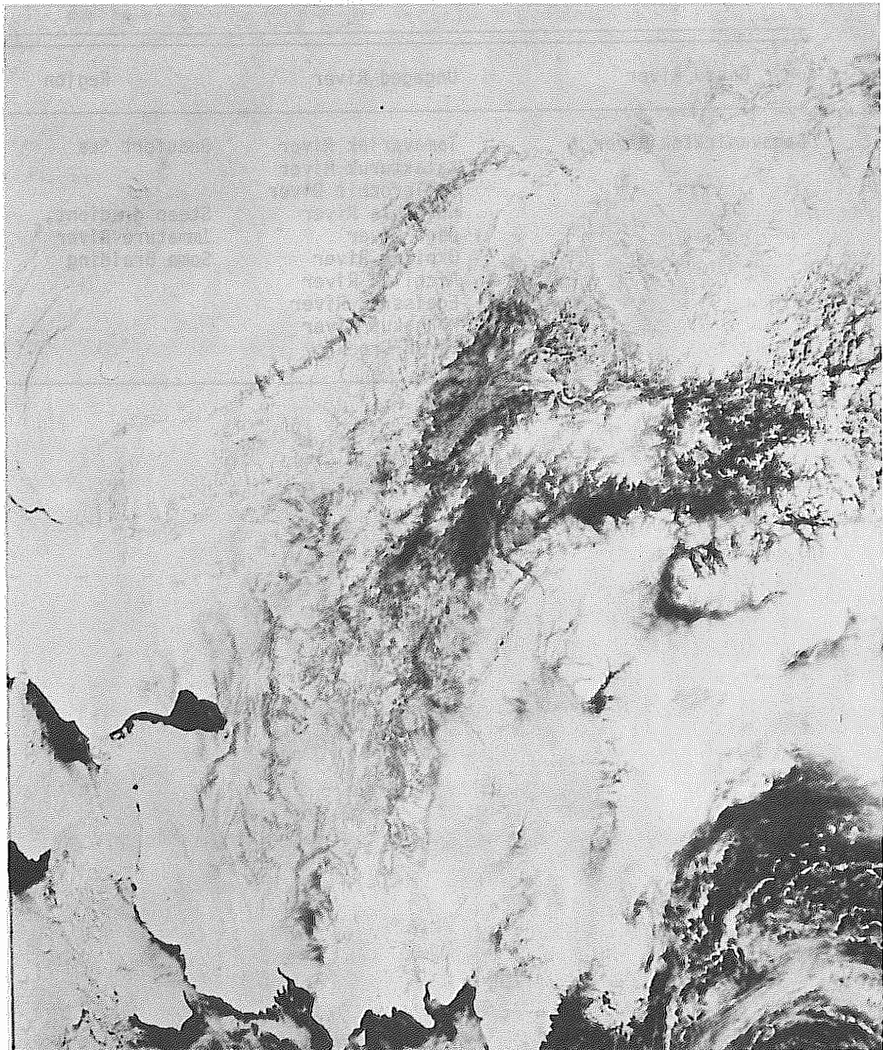
FIGURE 56: NOAA VISIBLE BAND IMAGE, ORBIT NO. 2093, May 1, 1975. This image depicts the earliest days of snowmelt. Unfortunately, the south coast is mostly clouded; however, the original darkening due to snowmelt is evident in the Tanana and Copper River Valleys.
