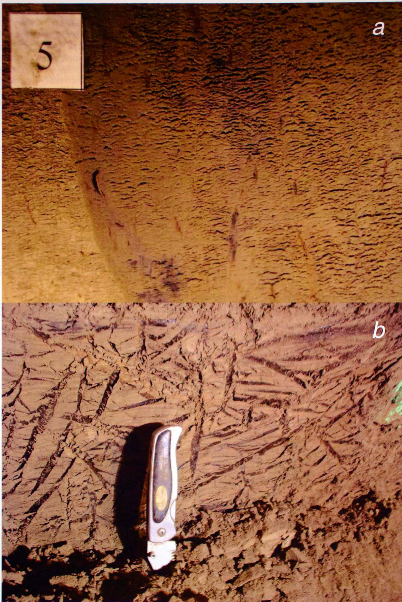
Figure 5. Photos showing (A) micro-lenticular cryostructure, location marker is 1.25 X 1.25 cm in size (photo by M. Kanevskiy), and (B) reticulate chaotic cryostructure, the handle of the knife is about 6 cm long (From Fortier et al. 2008).
