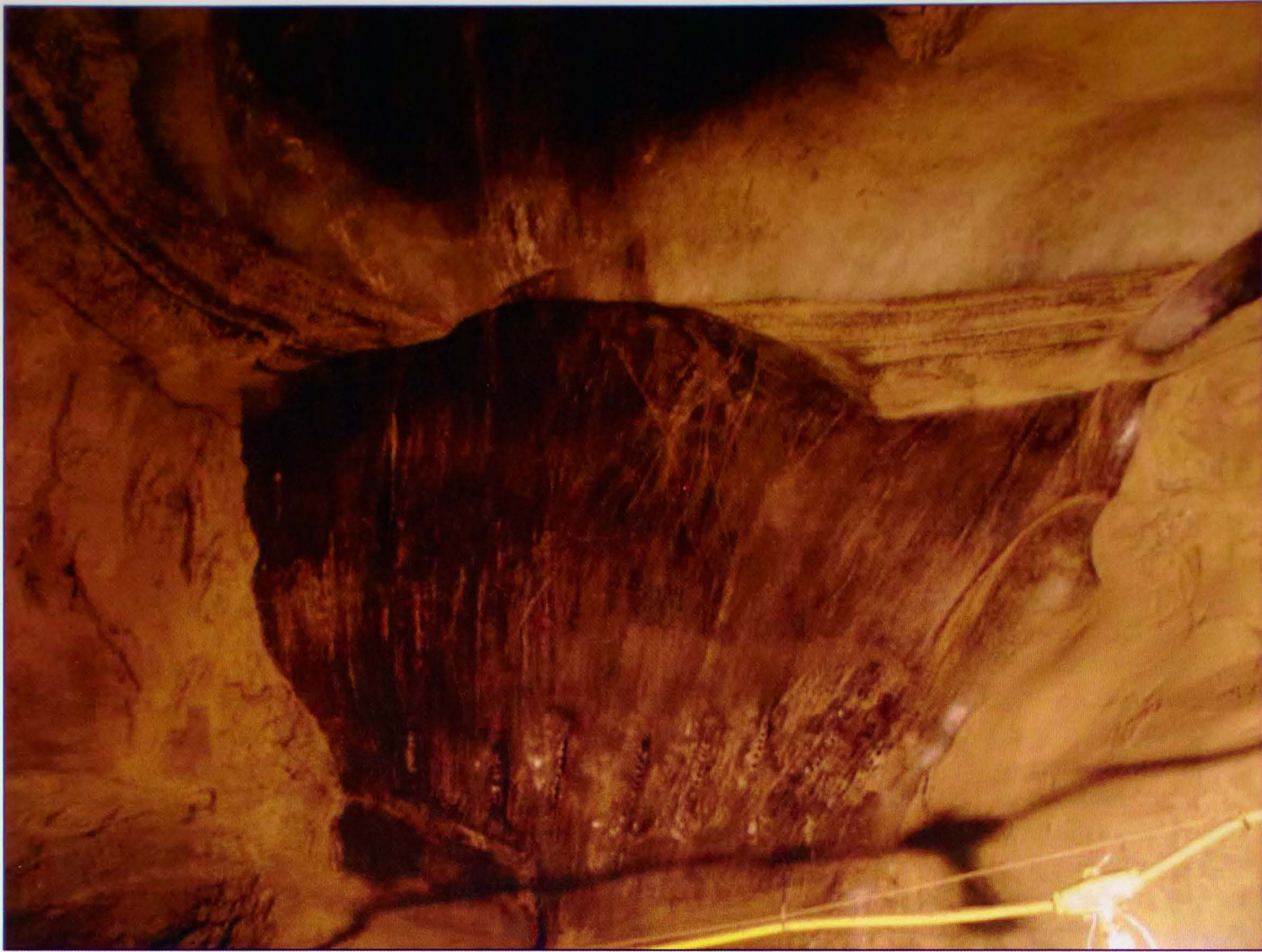
Figure 14. Photo showing ice wedge dissecting a horizontal lens of white thermokarst-cave ice (ice pseudomorph), right wall of the winze. The width of the wedge is 1.0 m. The thermokarst-cave ice body is underlain by several silt layers with reticulate-chaotic cryostructure. The same wedge exposed on the opposite wall of the winze is shown in Figure 12. (Photo by M. Kanevskiy).
