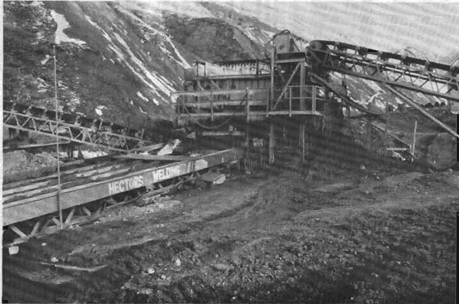
Fig 8: The El Jay screen is washed by 1,500 gallons of water per minute. The plus \frac{1}{4} " material is stacked (to the left) by another belt. The minus \frac{1}{4} " is then sluiced.
