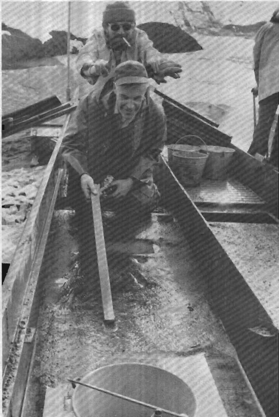
Fig. 13: Final stages of clean-up. The first separation is achieved in the box by paddling an even stream of water over the concentrate.
