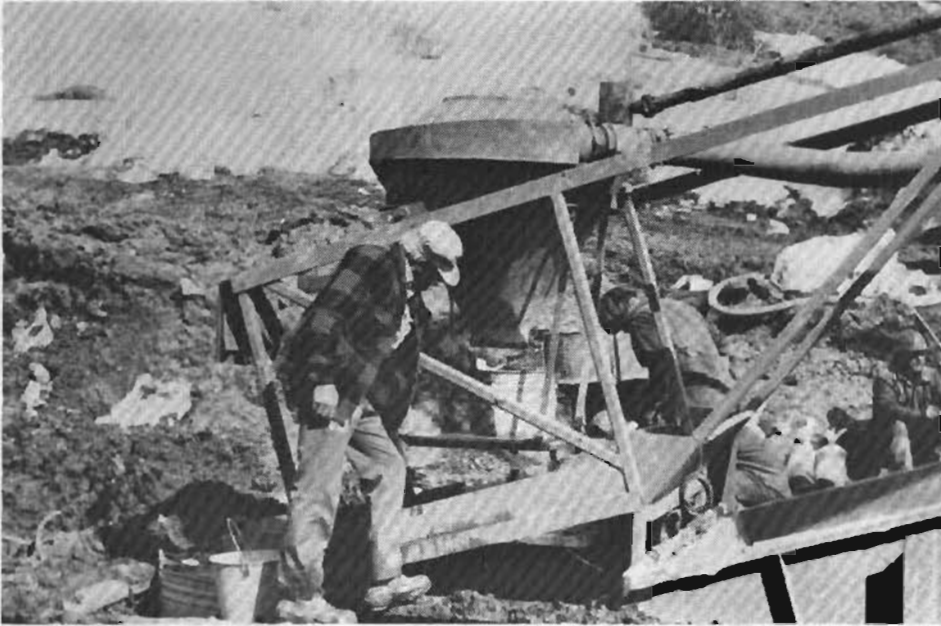
Fig. 3: The cyclone, with containers to catch the cuttings for volume measurements. Drilling is stopped at various intervals and the volume of the cuttings are measured for eventual comparison to the values of gold.
