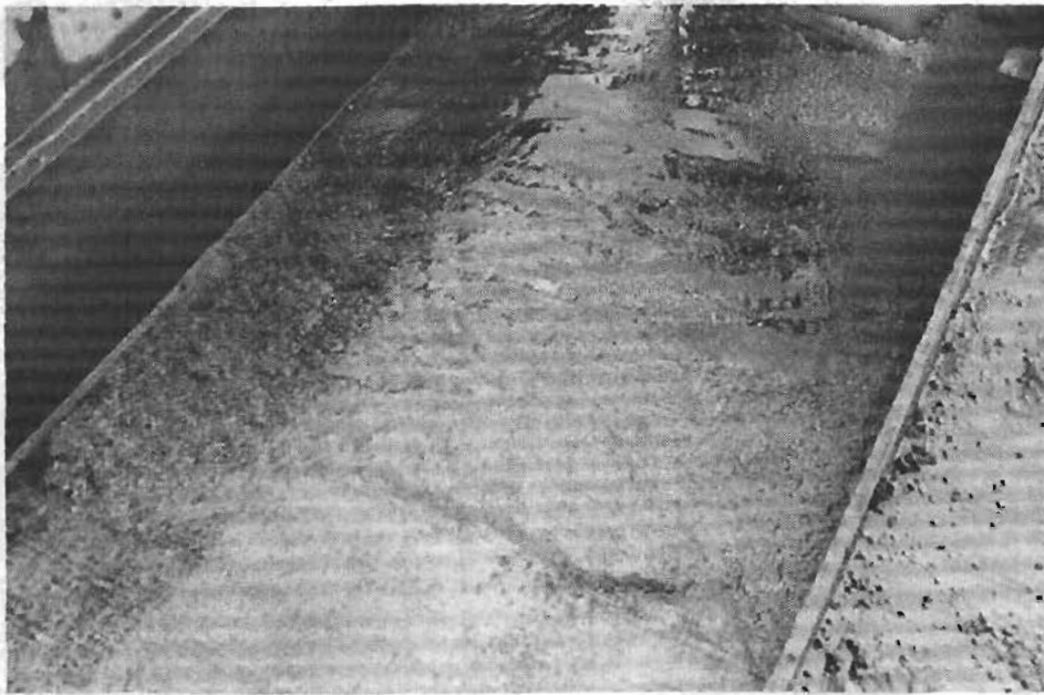
Fig. 14: Approximately 400 ounces, in one section of the box. An unusually good cleanup of -\frac{1}{2} " + 200 mesh gold.
