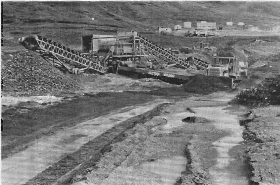
Fig. 11: Pushing fine tailings, the coarse ( +\frac{1}{2} " ) material accumulating at the end of the stacker belt will be moved next.
