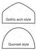
of structure is that the walls go straight up, allowing equipment such as rototillers or cultivators to work closer to the wall. The traditional Quonset style usually begins its curving arch right at soil level.
