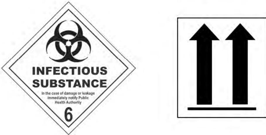
Figure 5. Safety marks for Category A infectious substances (10 cm x 10 cm or 5 cm x 5 cm) and orientation arrows indicate position of primary receptacles (size A7) ( Image adapted from WHO Guidance on regulations for the transport of infectious substances 2015–2016, WHO/HSE/GCR/2015.2, World Health Organization, Geneva, 2015)
