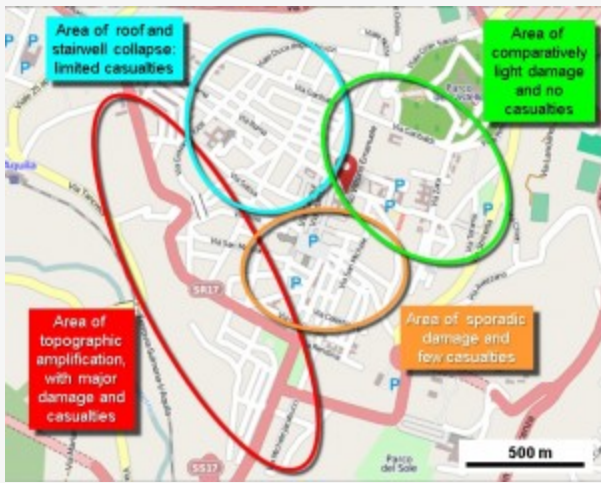
Fig. 9: Zones of building collapse in L'Aquila city centre.
