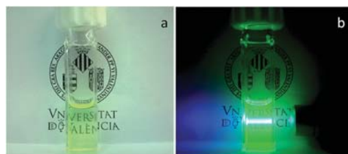
Fig. 1 Image of the toluene dispersion of CH 3 NH 3 PbBr 3 nanoparticles under (a) lab light and (b) UV-laser pointer excitation.
