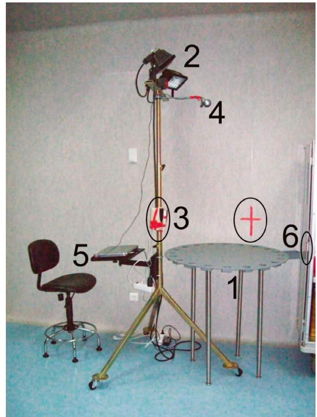
FIGURE 2 Barnes maze installation. 1. Barnes maze Table 2. Lights at the required high to achieve 3000 lux (lumen/m 2 ) on the Table 3. Speakers to apply 80 dB white noise during sessions. 4. Webcam. 5. Researcher location during sessions. 6. Scape tunnel (open), during each session it rests unseen under the table
