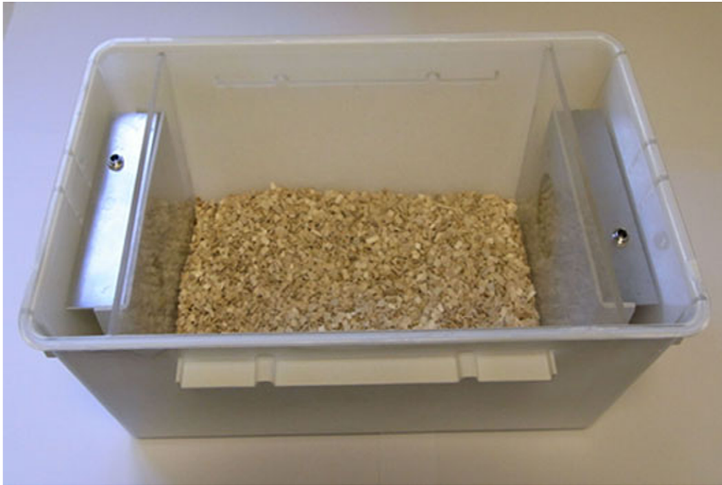
Figure 1. Cage for 670 nm exposure. LED lights were placed at both ends of the cage behind perspex screens. The internal space occupied a volume of 6,422 cubic centimeters (13 cm×26 cm×19 cm). A maximum of five animals were caged together. The longest distance the animals were from the light source was approximately 13 cm and the minimum was 0.4 cm, which is the thickness of the perspex screens. doi:10.1371/journal.pone.0057828.g001
