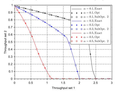
**Figure 6.** Throughput region of a multi-packet reception (MPR) system with two subsets of terminals:  $J_1 = 3$  and  $J_2 = 1$  using the general reception model with different values of the reception parameter  $\alpha$ .
