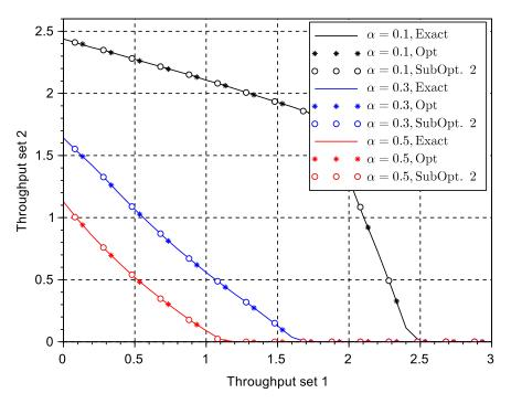
**Figure 5.** Throughput region of a multi-packet reception (MPR) system with two subsets of terminals:  $J_1 = J_2 = 3$  using the general reception model with different values of the reception parameter  $\alpha$ .
