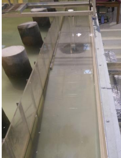
Figure 4.46 – Downstream view of the wave flume (wave tank corridor) with the model of the monopile placed at the center [157].
