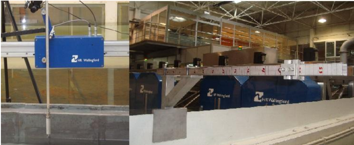
Figure 4.53 – 2D bed profiler mounted on the longitudinal rail (left) and ruled cross-sectional rail used to guide the profiler in the measurement grid.
