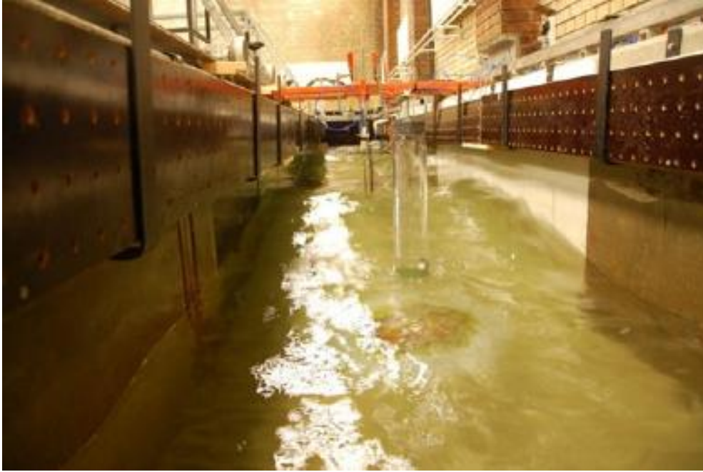
Figure 4.8 – Testing in the wave-current flume with the protected monopile present [102].
