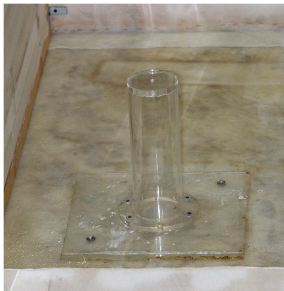
Figure 4.49 – Monopile base and transition piece at 40 cm height.
