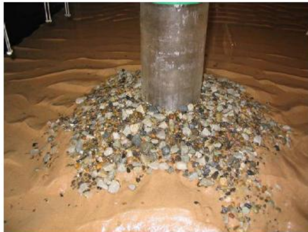
Figure 3.32 – Physical model of a damaged scour protection around a monopile from [169].
