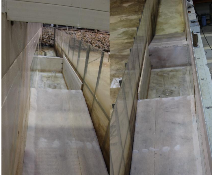
Figure 4.48 – Upstream view (left) and downstream view (right) of the approaching slopes and the sediment box, before the sand bed installation.
