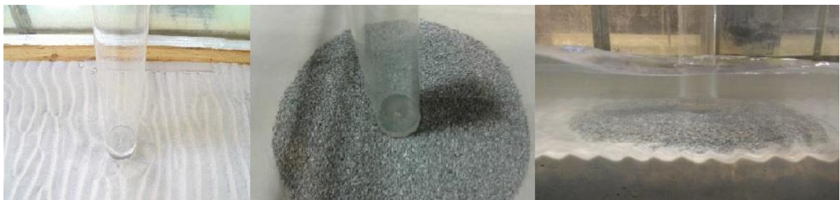
Figure 4.51 – Model of the monopile foundation: during testing without protection (left), before testing with protection (center), during testing with protection (right).
