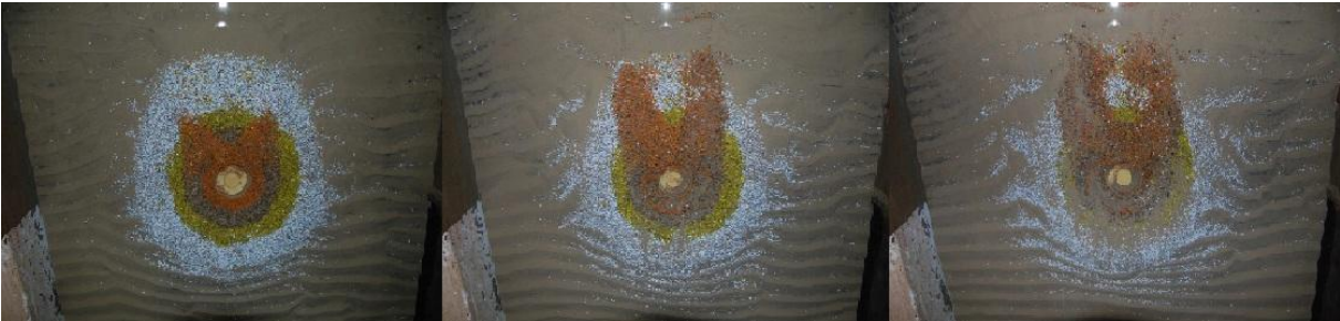
Figure 4.32 – Evolution of the V-shape form registered during s1_005: left – after 1000 waves, middle – after 3000 waves, right – after 5000 waves. Flow direction from the bottom to the top.
