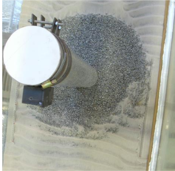
Figure 4.52 – Monopile and scour protection models after a test.
