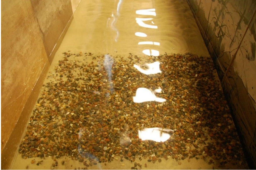
Figure 4.4 – Sand gravel placed on the upward slope to reduce turbulence and smooth the boundary layer.
