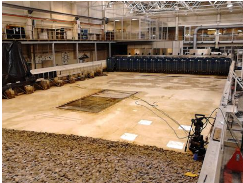
Figure 4.45 – Wave tank view from the downstream side, at the absorbing beach, towards the multi-element wave paddles.
