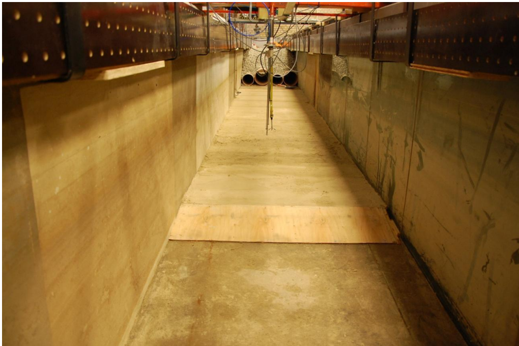
Figure 4.5 – Downstream view of the bypass section, wave gauge and ADV, without the monopile present.
