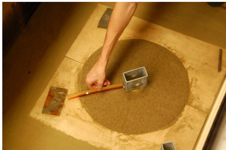
Figure 4.10 – Granular filter layer being placed beneath the armour layer stones.
