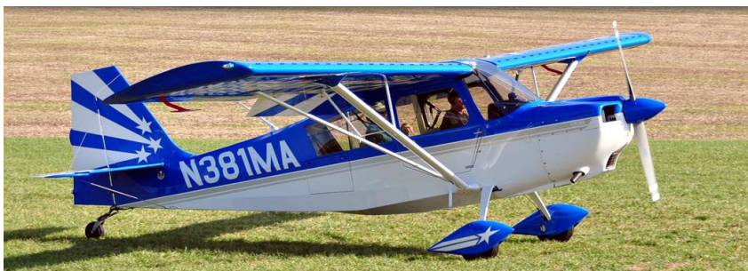
Figure 3.3 - Citabria Explorer with NACA 4412 profile on the wings [27].
