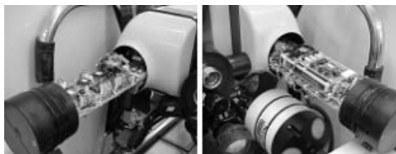
Fig. 1. On the left the starboard cylinder with an electronic compass and the dimmer and motor controllers. On the right the port cylinder with the on-board power supply system and also it's monitor.
