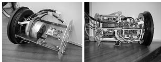
Fig. 2. On the left the inertial system and on the right the PC104 CPU stack
