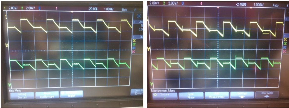
Figure A. 5- TXP (yellow signal) and TXN (green signal) signals obtained, when the sensor is connected, from the developed prototype extension (left image) and from the board with a new configuration (right image).
