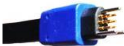
Figure 3.7.1- Programming connector used to program the microcontroller in the module. This connector has six connections with spring connector and three metal guides to help in the connector positioning in the board. It is developed by Tag-Connect and the other side of the cable is an internet connector (RJ12 connector) that plugs directly to ICD-3, which is the programmer used in this work. [97]
