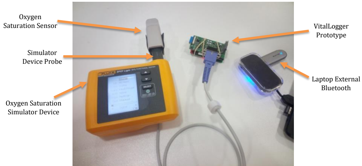
Figure 3.5.1- This image shows the FLUKE simulator device and the prototype during the calibration process. The prototype was connected with a laptop through a Bluetooth connection, sending the calculated R values.
