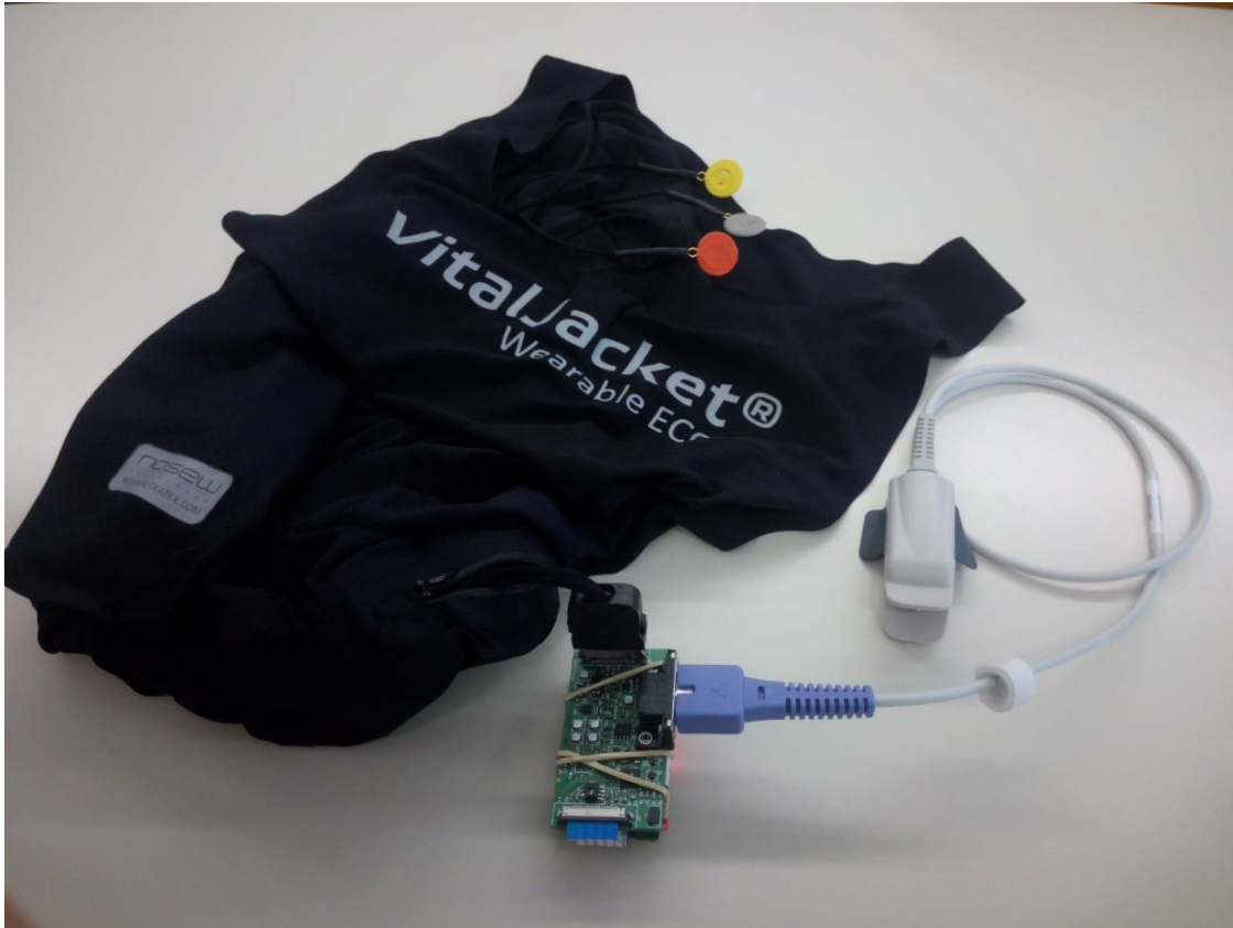
Figure 3.6.1- Final developed VitalLogger prototype system with the following sensors: electrocardiogram (ECG) and heart rate and tri-axis accelerometer from the main board and oxygen saturation percentage and ambience temperature and relative humidity from the developed extension board.
