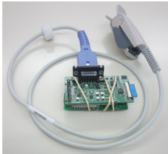
Figure 3.3.13 - VitalLogger first prototype connected to the main board and with the Oxygen Saturation sensor plugged in.
