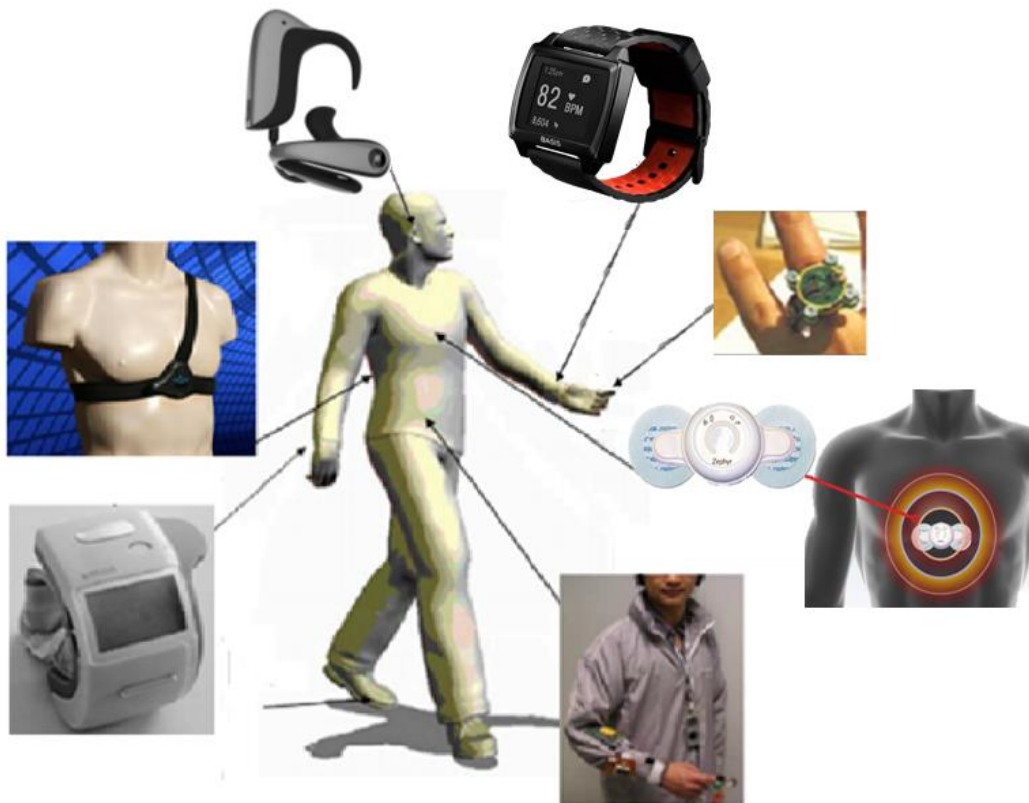
Figure 2.2.1- Examples of wearable medical devices and prototypes. From the top in clockwise: a new ear prototype to measure several physiological parameters; smartwatch Basis PEAK™ [21]; a finger ring prototype for plethysmography; an ECG BioModule (BioPatch™) attached to normal electrodes in the chest [22]; a prototype jacket with several sensors; a wrist-worn device (AMON); and a chest belt to measure respiration rate and ECG (Bmedical®). Adapted from [4, 23, 24]
