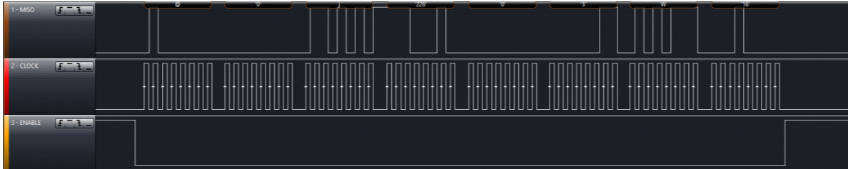
Figure 3.4.17- SPI digital acquisition of the HIH6130 reading process. First 32-bit represents the temperature reading and the remaining 32-bit represents the relative humidity reading.
