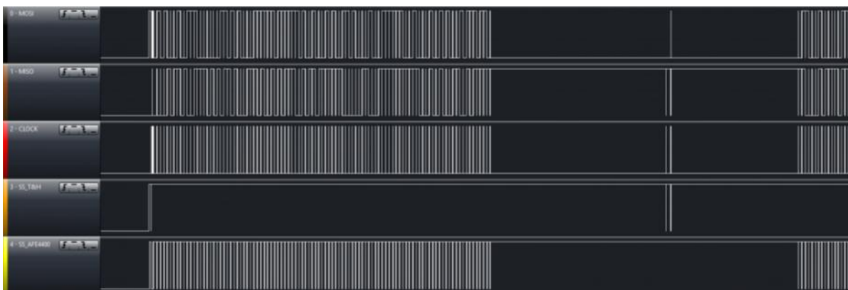
Figure 3.4.3- SPI digital acquisition of the first cycle including the initialization. First it is visible a higher density of SPI communication which represents the initialization referred above. Then a reading until 100 samples it’s made. The following space without communication corresponds to the time where the oxygen saturation value is computed and then an ambience temperature and relative humidity reading is performed. It is still possible to view the start of a new reading, without the initialization process.
