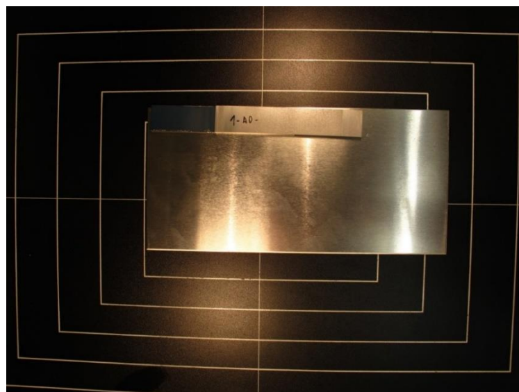
Figure 47 - Comparison of the initial dimensions and final dimensions of the specimens to be tested with 230x110x2 mm for the bigger plate.
