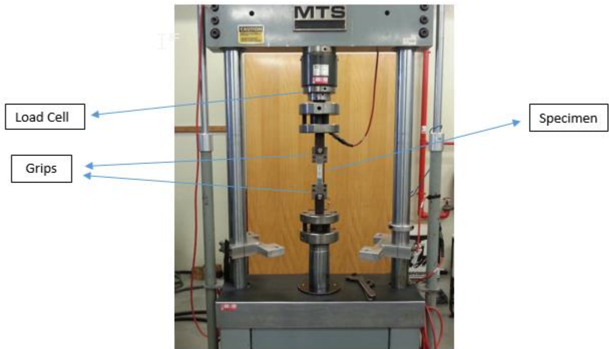
Figure 66 – MTS Landmark Servo hydraulic Test Systems used to perform the fatigue tests.
