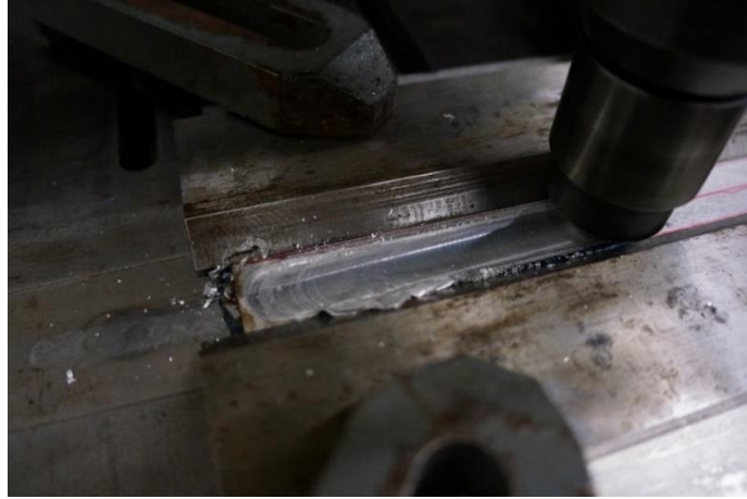
Figure 52 - FSW pin welding the bonded joint.
