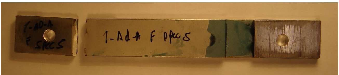
Figure 68 - Failure of the aluminum on the adhesive SLJ.
