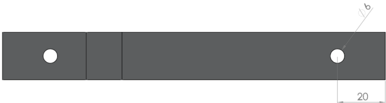
Figure 67 - Schematic of the clamping configuration (not to scale) for fatigue tests with: a) front view and b) upper view.
