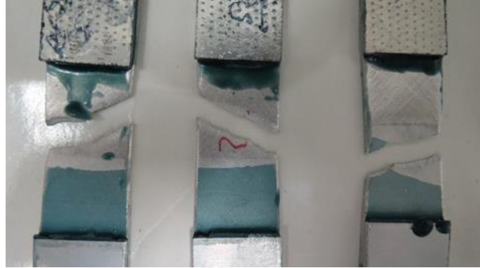
Figure 92 - Failure on SLJ specimen AD-A.
