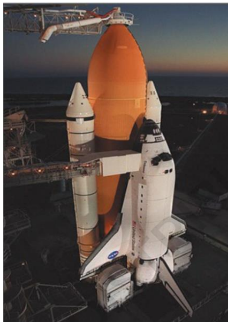
Figure 7 - Space shuttle and the external fuel tank [13].
