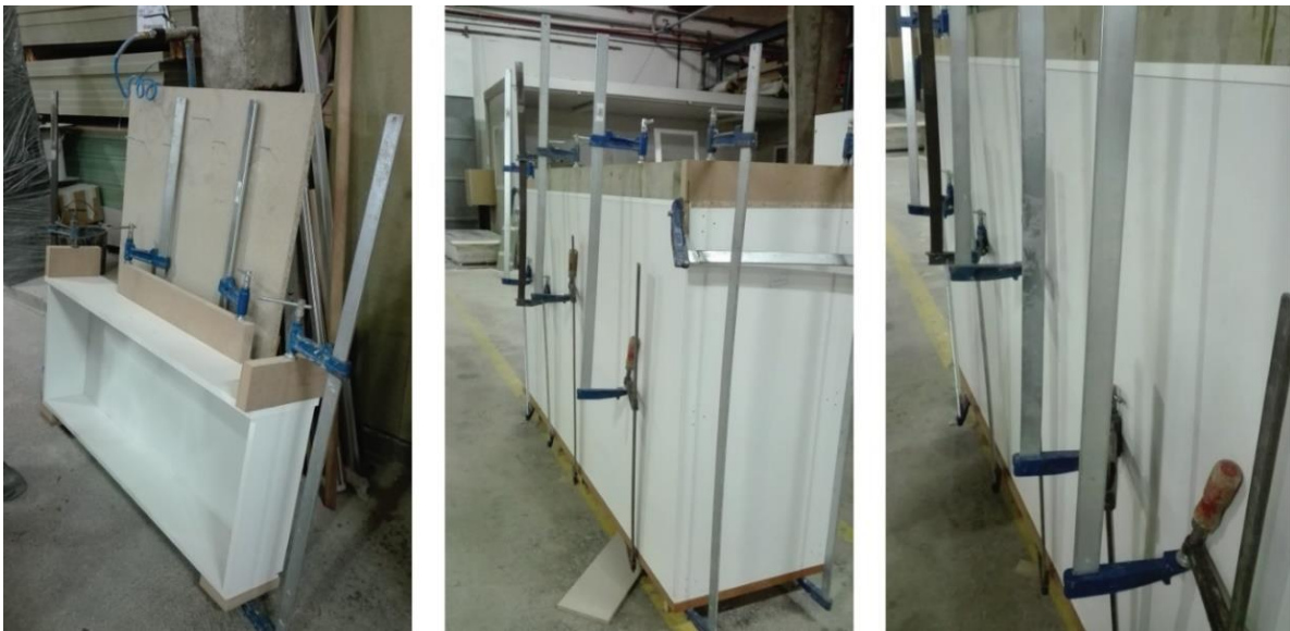
Figure 48 – Assembly of a drawer fixed with wood dowels and glue at CarpinCasais.
