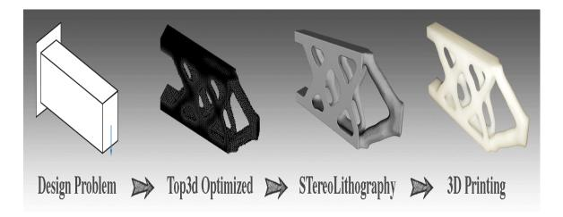
Fig. 5.30. Topology Optimized Structure
