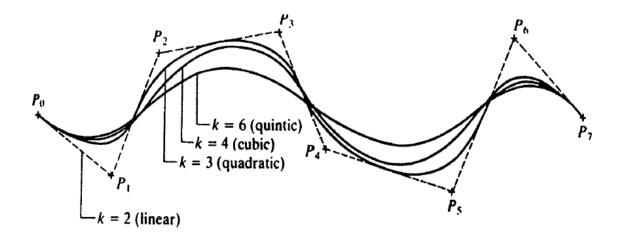
Fig. 2.6. B-Spline Curve with degree variation
