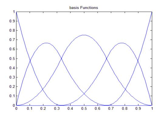
Fig. 3.4. Basis Function for order, k=3 which are parabolic paths
