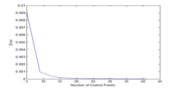
Fig. 5.19. (c) Error Vs Number of Control Points for Involute gear profile
