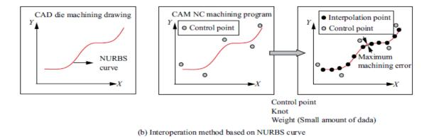
Fig. 2.17. Comparison between line segment and NURBS interpolation
