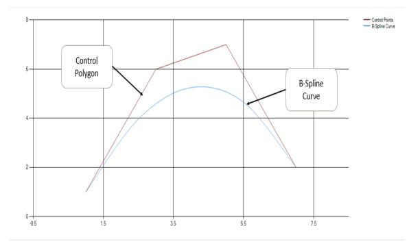
Fig. 2.7. Example of B-Spline Curve
