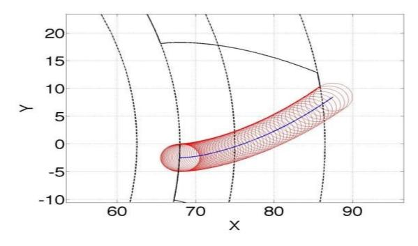
Fig. 5.16. (b) Involute Gear Profile of a single tooth
