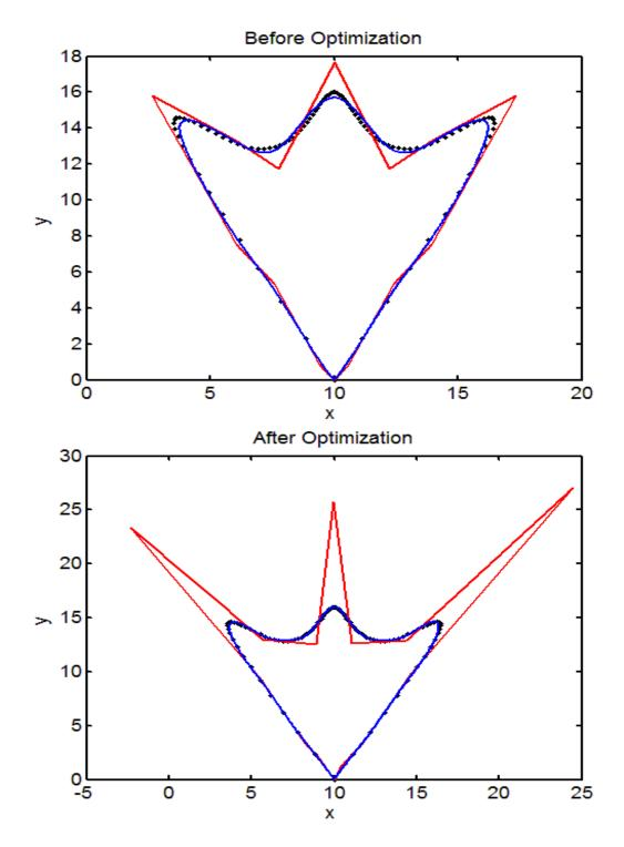
Fig. 4.12. Comparison of the approximate NURBS curve before optimization and after optimization for Trident Curve.
