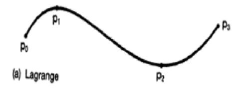
Fig. 2.1. Lagrange interpolation of a curve
