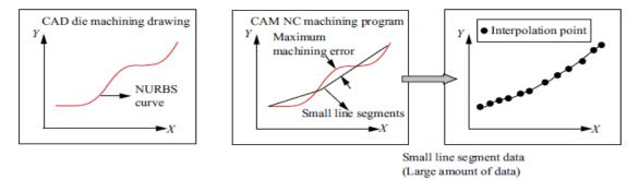
(a) Interoperation method based on small line segment approximation
