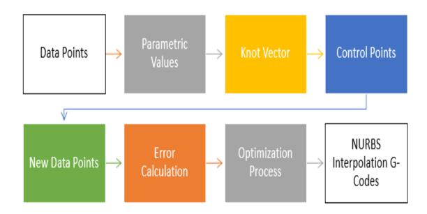
Fig. 5.1. NURBS function block diagram
