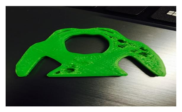
Fig. 5.36. Topological optimized structure developed using 3D printer with NURBS optimal parameters
