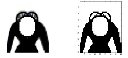
Fig. 5.31. (a) Topology optimized structure and (b) Topology optimized structure with pixel values 0s and 1s
