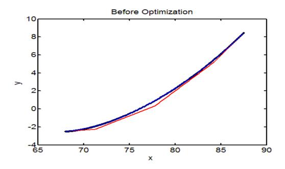
Fig. 5.17. (a) Involute gear profile before optimization using NURBS function
