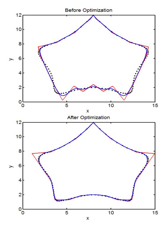
Fig. 4.11. Comparison of the approximate NURBS curve before optimization and after optimization for Star Shape.
