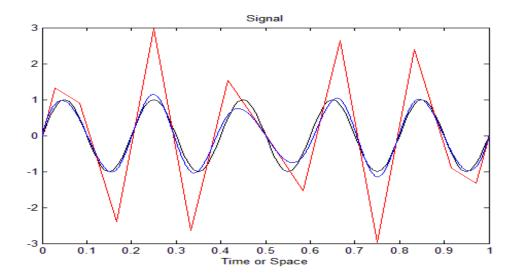
Fig. 3.6. Plots of Data points curve (black), control points polygon (red) and approximate NURBS curve (blue)
