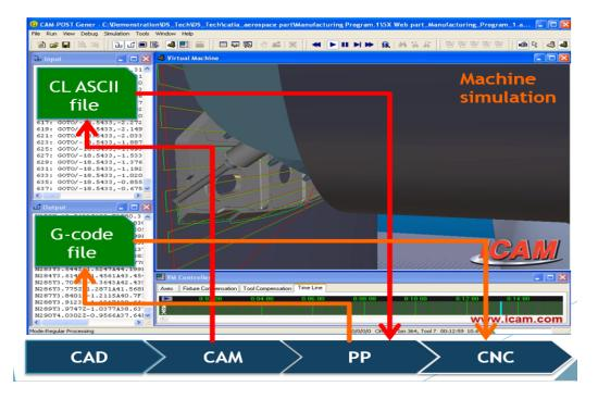
Fig. 1.2. CNC Part Programming workflow
