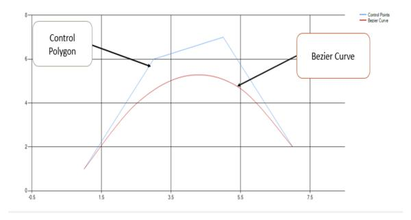
Fig. 2.5. Example of Bezier Curve
