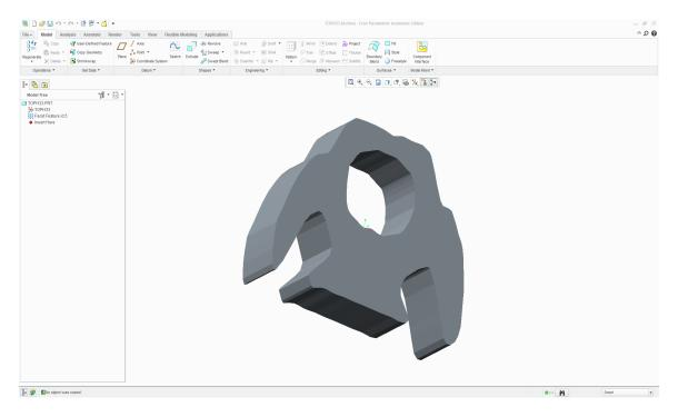
Fig. 5.35. Topological optimized structure developed using Pro-E software with NURBS optimal parameters
