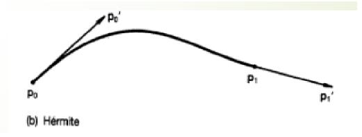
Fig. 2.2. Hermite interpolation of a curve
