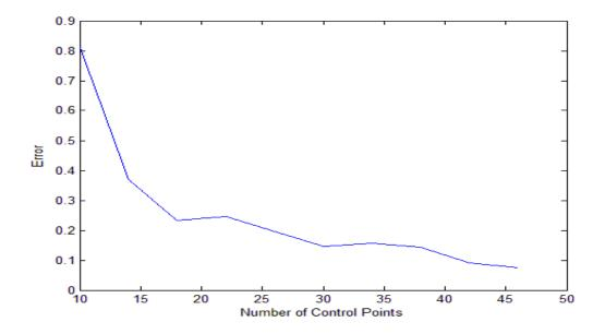
Fig. 5.8. Error Vs Number of Control Points for Star Shape curve
