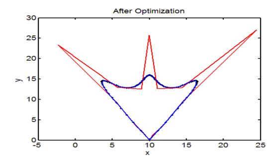
Fig. 5.11. Trident Curve using NURBS after optimization
