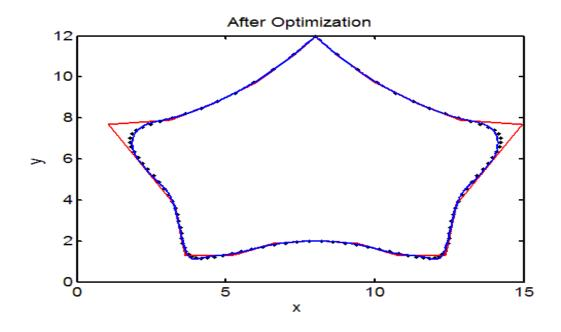
Fig. 5.7. Star Shape curve using NURBS after optimization
