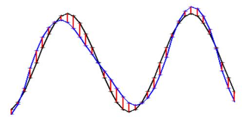
Fig. 3.8. Truncated View of error between the data points curve and the approximate curve
