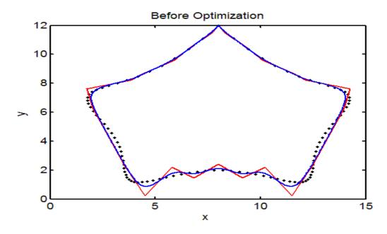
Fig. 5.6. Star Shape curve using NURBS before optimization
