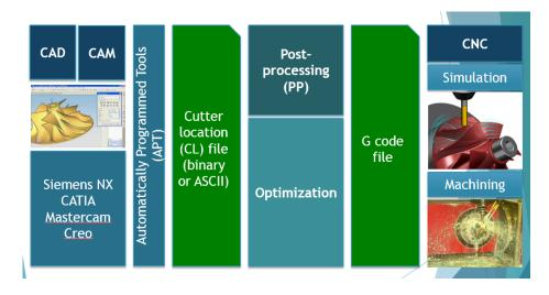
Fig. 1.1. Optimized Process workflow for CNC machining
