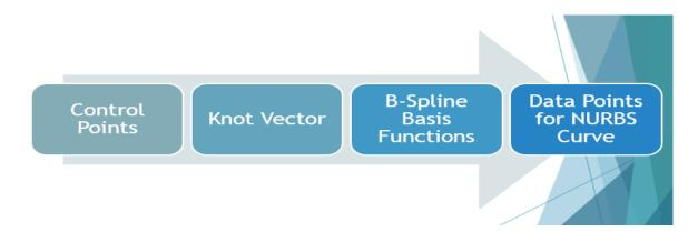
Fig. 2.9. Block diagram of NURBS formulation
