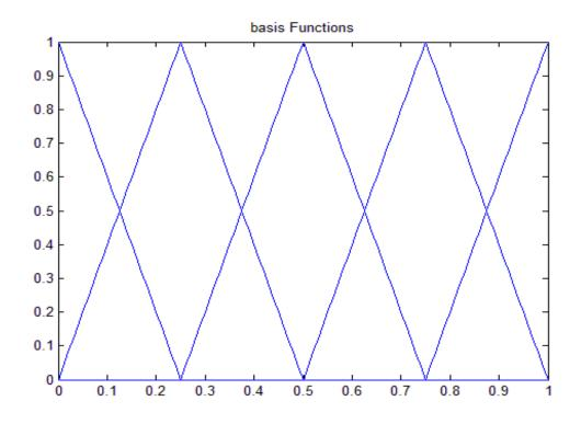
Fig. 3.3. Basis Function for order, k=2 which are straight lines
