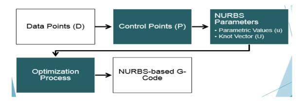
Fig. 3.1. Block diagram for NURBS function methodology
