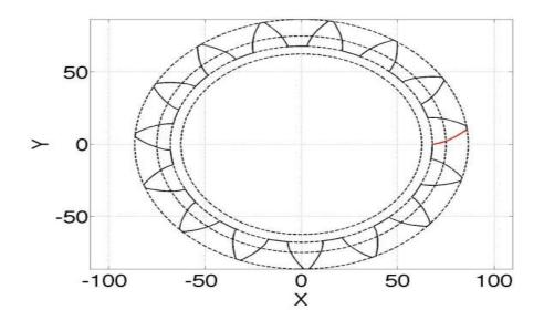
Fig. 5.15. (a) Complete Involute Pinion Gear Profile
