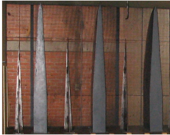
Figure 1. Vortex generators (Irwin and Counihan spires) located at the beginning of the flow development zone
