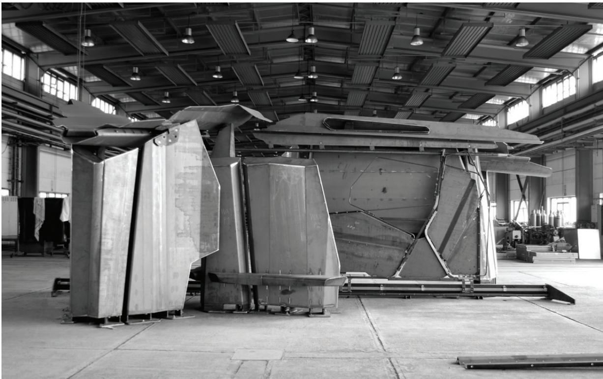
Fig 5.3.10 Manufacturing Protoarchitecture 2: The fully assembled '55/02' shelter at the factory of Stahlbogen GmbH in Blankenburg, prior to dismantling, finishing and delivery to site. Material: Steel.
