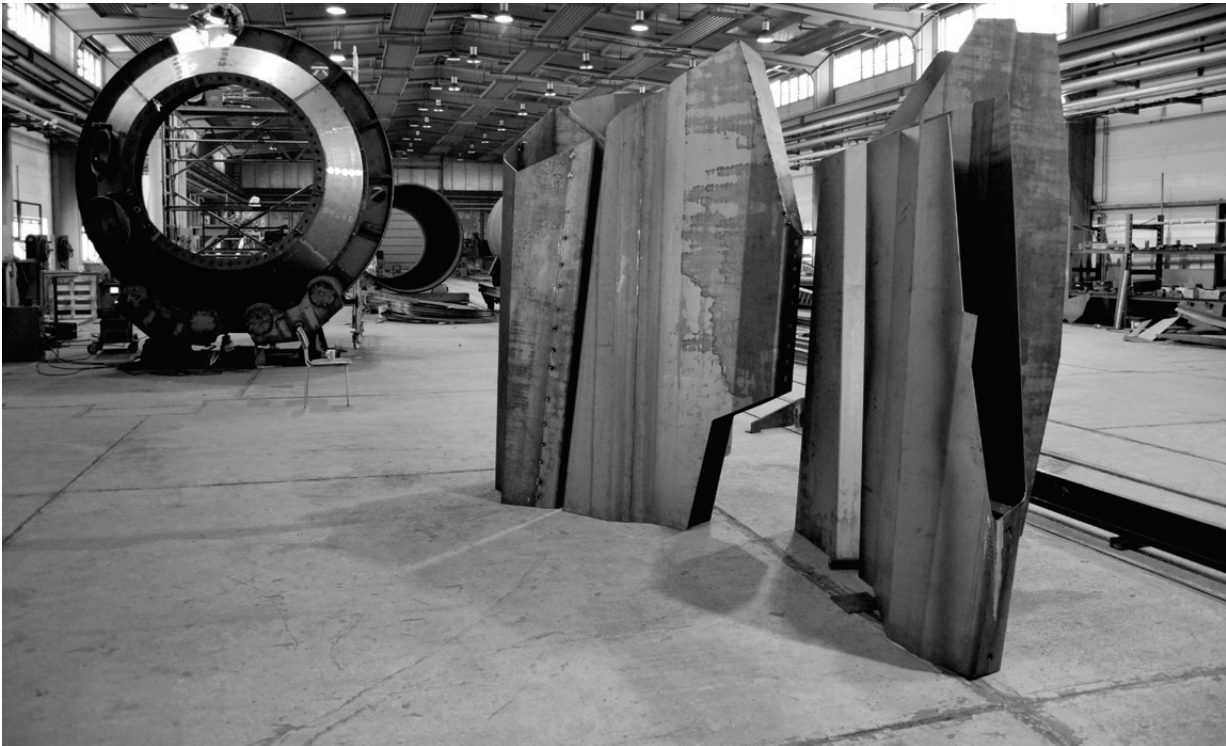
Fig 5.2.1 Manufacturing Protoarchitecture 1: In the foreground, early components of the '55/02' shelter by sixteen*(makers) in collaboration with Stahlbogen GmbH. In the background components of more everyday fabrications by Stahlbogen. For the former, precise assembly of the digital model was not a project objective, for the latter, it is a quality upon which the business depends. Material: Steel
