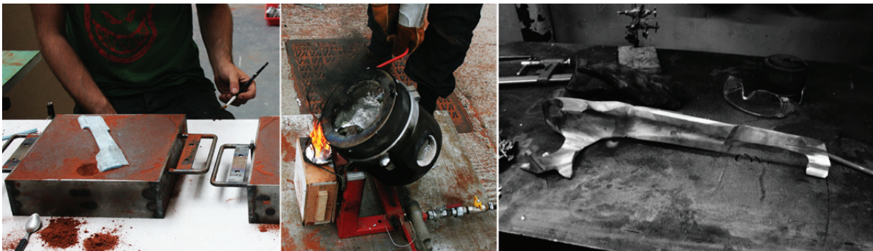
Fig 5.3.5 Incisions in the Haze from the Prosthetic Mythologies project by Kate Davies and Emmanuel Vercruyssen of LiquidFactory (2012). The alchemy of the sand casting is magical. The foam form is buried in sand, packed down and engulfed in its cocoon, molten metal is poured into it, dissolving and replacing the foam - transfiguring it - when the form boxes are opened a fiery hot object shrouded in smoking burnt black sand emerges. Materials: Sand, Aluminium, Gas.
