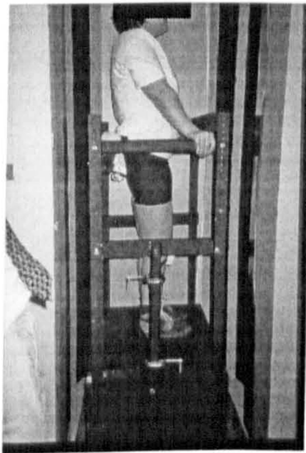
Figure 1. A paraplegic stands in the Oswestry frame inside the scanner. The scanner heads are located at the front and back of the scanner, consequently this design of frame has very little structure in the viewing fields of the heads over the required area, the legs.
