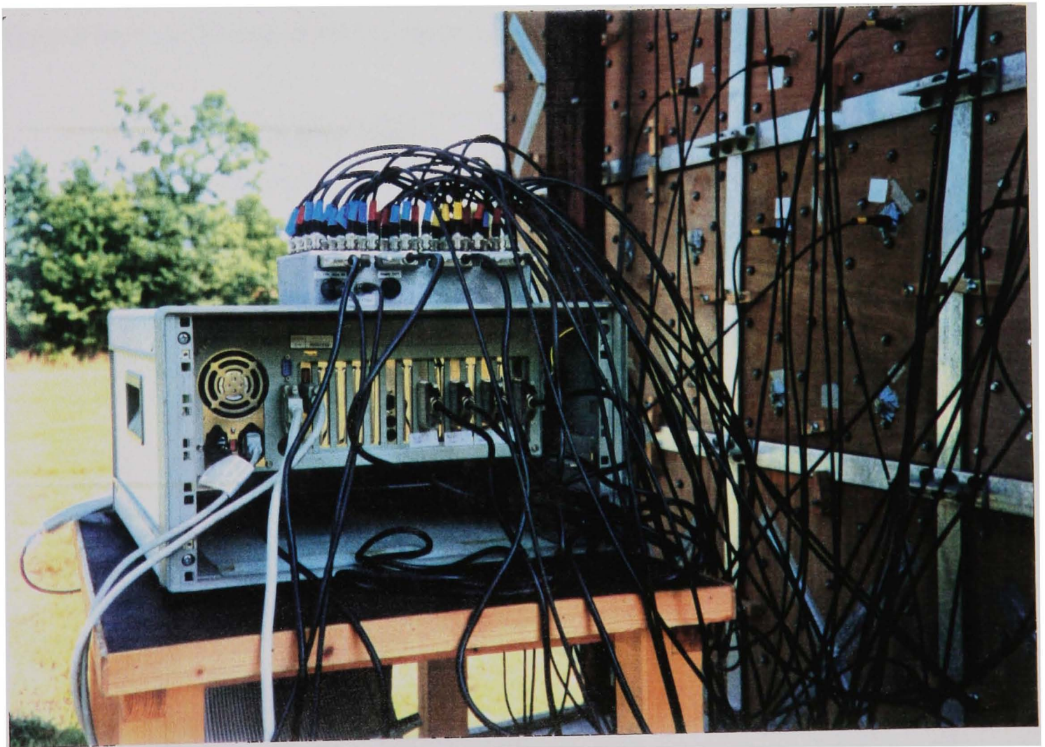
Figure 2.25 The connection to the data acquisition boards for multiple-channel measurements.
