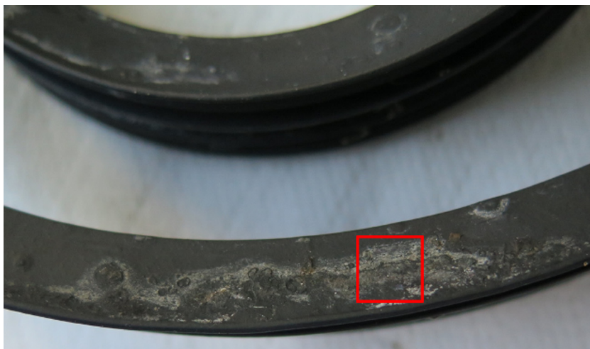
FIG 1 Biofilm formed on rubber seals in residential DWs. Microbial biofilm formation on DW rubber seal; the square (in red) represents the 1-cm 2 sampling site. Biofilm samples from 1 cm 2 were collected by scraping the surface of rubber seal with a sterile scalpel for DNA extraction and further analysis. Sampling was done in situ , with the seal at its original place.
