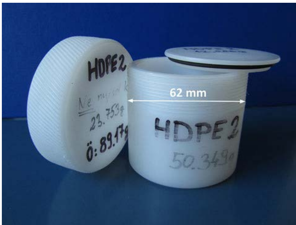
Figure 9. The sample container made of HDPE (High-density Polyethylene) and Viton O-ring.
