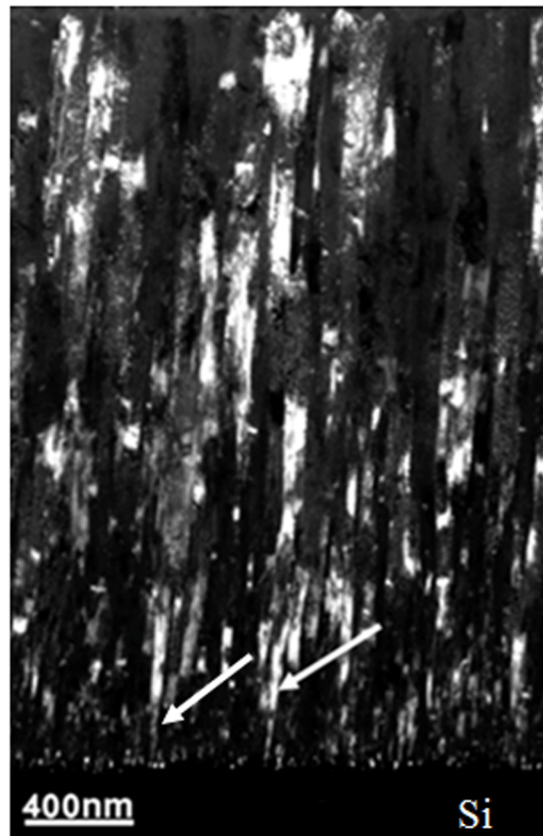
Figure 5.4. Dark field X-TEM image of the undoped TiN film taken by the 111 TiN reflection the crystals marked by arrow demonstrate the V-shaped morphology of the \langle 111 \rangle oriented crystals in the thickness domain near to the substrate.
