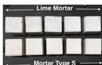
Figure 1. Red-Green-Blue (RGB) image of mortar samples across the two mortar classes
