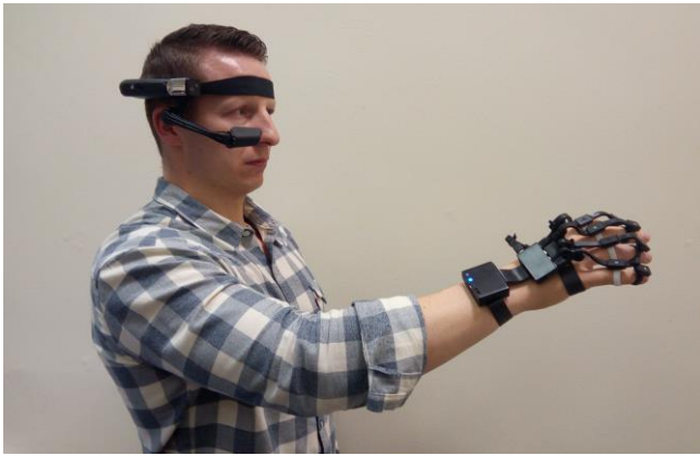
Fig. 6: System Implementation: User with HMD and VR Glove
