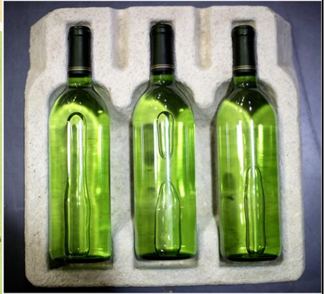
The design company Ecovative makes a variety of packaging materials using mycelium fungus. Nathaniel Brooks for The New York Times
