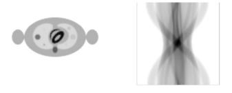
FIGURE 3.6: During the 2D PET acquisition, the object emitting radioactivity on the left-hand side provides the sinogram on the righthand side.
