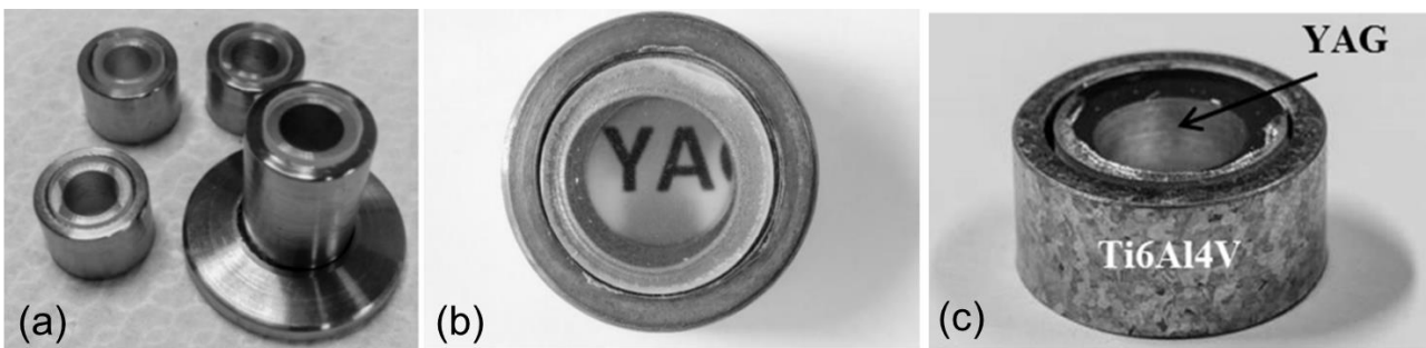
Figure 6.39. Ti6Al4V pipe used for the optical window substrate prototype (a); top view (b) and lateral view (c) of the YAG/Ag/Ti6Al4V joining sample.
