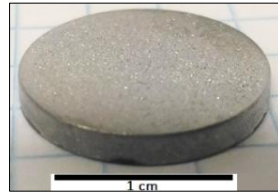
Figure 6.66. The Al_{84}Ti_{16}/SiC sample after the wetting test at 1300°C (10 min).
