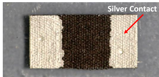
Fig. 3.1. Sample for sheet resistance measurement with 5 \times 5 \text{ mm}^2 surface area. Highly conductive silver paint was used to make contacts of 5 \times 2.5 \text{ mm}^2 size on both ends.
