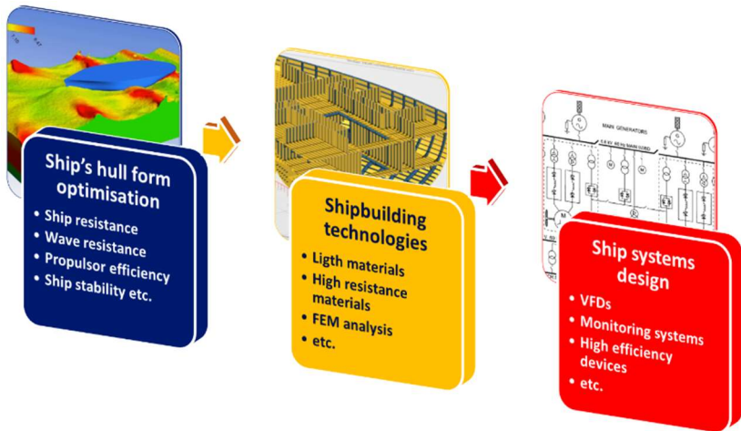
Figure 51 - Areas of action to improve ship's energy efficiency
