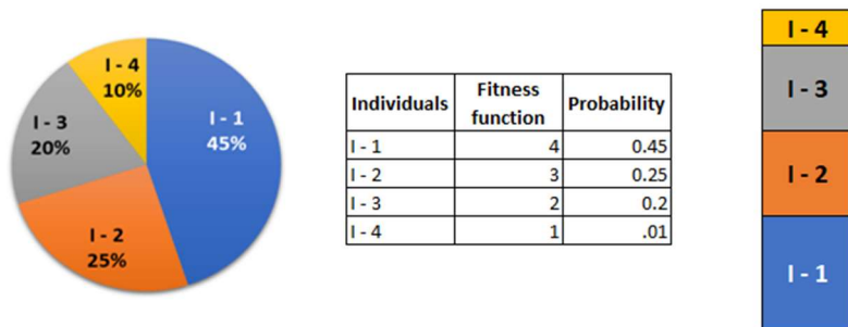
Figure 57 - Genetic algorithms crossover roulette wheel approach
