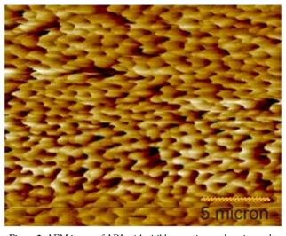
Figure 2: AFM image of APA with visible pore size on the microscale.
