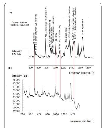
**Figure 5: (A)** Reference lysozyme Raman spectra with the peaks assignment obtained by our group in 2014 [21]; **(B)** Raman spectra of CFSE-labeled lysozyme, incorporated in the APA pores.
