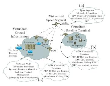
Fig. 2. Road-map for an SDN/NFV-enabled satellite network
