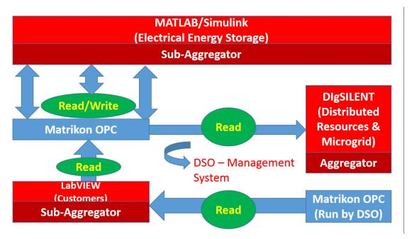
Figure 1: Proposed Architecture for Virtual Power Plant
