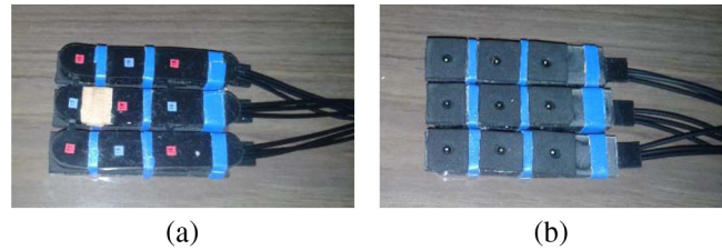
Fig. 1 Silicon probe use for the measurements on the neonates' heads. Red squares: injection points; blue squares: detection points. (a) External side and (b) surface in contact with the head (fiber tips are visible).
