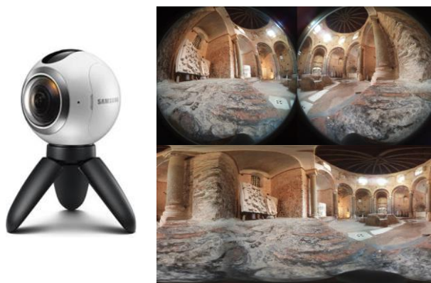
Fig. 1. The Samsung Gear 360 and its two circular images (top) turned into a single equirectangular projection (bottom).
