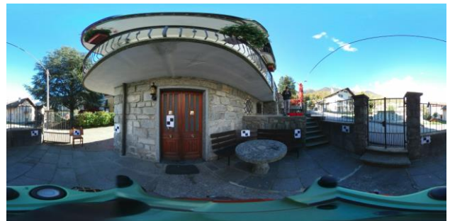
Figure 5. One of the equirectangular projections and the 8 targets used as control and check points.
