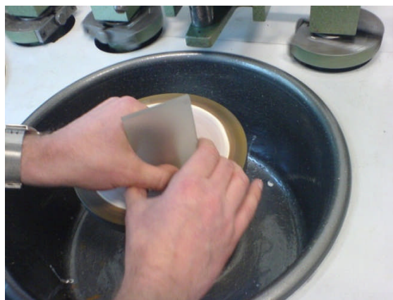
Figure 6.26: Waveguide end facet roughness hand polishing
