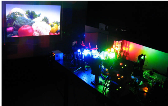
Figure 3.1: The laser projector demonstrated by Barco Technology[3.5]. The picture in the top left corner in the image is projected by a laser based projection system.
