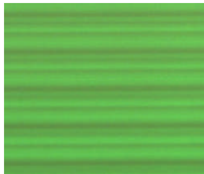
Figure 8.2: The recorded pattern of the scanned line after using free space homogenisation of the NECSEL laser beam
