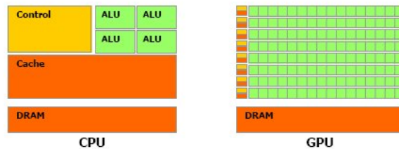
Figure 5.1: Diagrammatic representation of single core CPU architecture and GPU. Whereas CPUs have layers of cache and optimised execution, GPUs favour increased compute capacity. (image credit: Nvidia [20])
