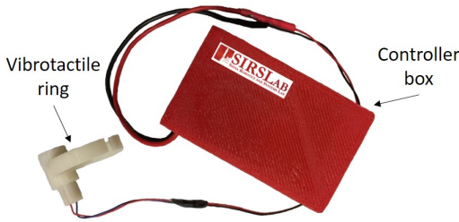
Fig. 4: Vibrotactile ring with its controller box. During the experiments the ring is worn on the operator’s left hand and the box is attached to a Velcro bracelet worn on the forearm. message is the same, i.e. , informing in a reactive way the human that the robot has understood his/her intention and is about to move.
