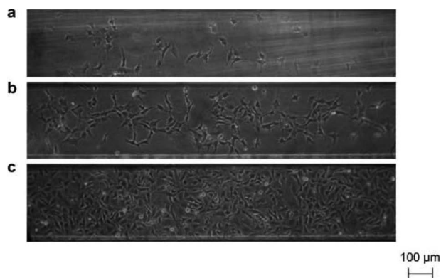
Fig. 4 Image of cells cultured in the microchip. (a) Polystyrene (PS) microchip, 1.3 \times 10^6 cells/mL; (b) PS microchip, 2.6 \times 10^6 cells/mL; (c) PS microchip, 7.0 \times 10^7 cells/mL.
