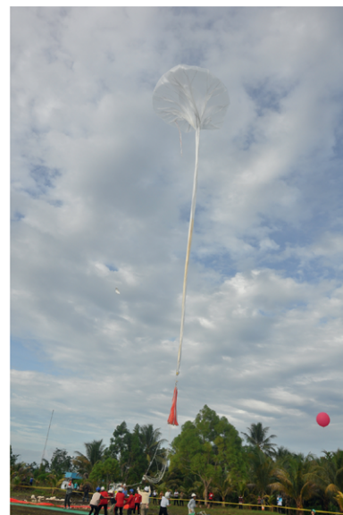
FIG. 9. (left) Stages of the launch procedure. (a) The balloon bottom is held by an anchor during gas inflation. (b) After gas inflation, the balloon is raised by opening the spool and removing the safety rope. (c) The collar is released. (d) The balloon is launched by cutting the anchor rope. (right) A snapshot showing the balloon launch for cryogenic air sampling at Biak on 24 Feb 2015.
