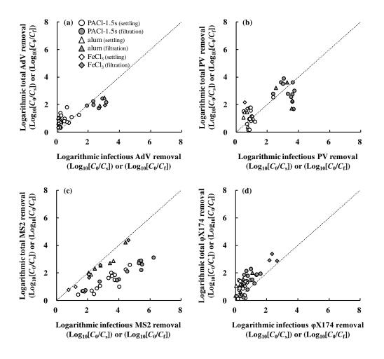
Figure 9. Comparison of infectious virus removal ratios evaluated by the PFU method and total virus removal ratios evaluated by the PCR method for AdV (a), PV (b), MS2 (c), and  $\phi$ X174 (d) during coagulation.
