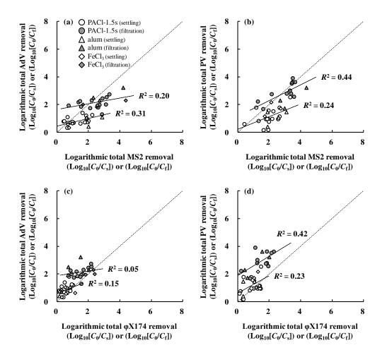
Figure 6. Relationships between total AdV and MS2 removal ratios (a), total PV and MS2 removal ratios (b), total AdV and φX174 removal ratios (c), and total PV and φX174 removal ratios (d) during coagulation.
