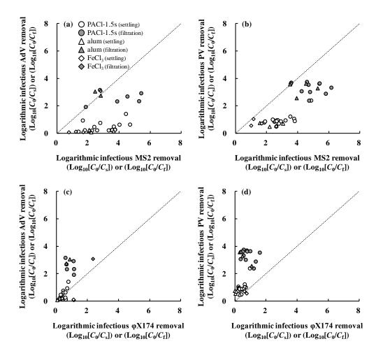
Figure 5. Relationships between infectious AdV and MS2 removal ratios (a), infectious PV and MS2 removal ratios (b), infectious AdV and φX174 removal ratios (c), and infectious PV and φX174 removal ratios (d) during coagulation.
