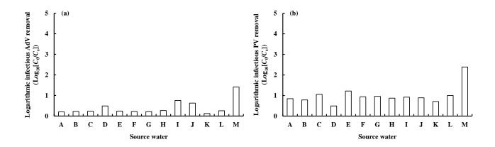
Figure 1. Effects of source water quality on removal of infectious AdV (a) and PV (b) by coagulation with PACI-1.5s and settling, as evaluated by the PFU method.
