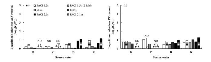
Figure 3. Effects of coagulant dosage and coagulant type on removal of infectious  ${\rm AdV}\left(a\right)$  and
