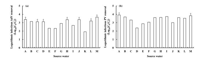
Figure 2. Effects of source water quality on removal of infectious AdV (a) and PV (b) by coagulation with PACI-1.5s, settling, and filtration, as evaluated by the PFU method. Arrows indicate that the virus concentrations were below the quantification limit (1/6 PFU/mL).
