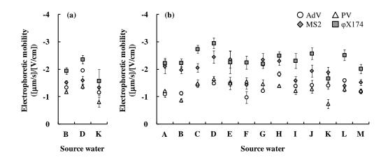
Figure 7. Electrophoretic mobilities of AdV, PV, MS2, and  $\varphi$ X174 in filtered source water
