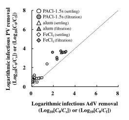
Figure 10. Relationship between infectious PV and AdV removal ratios during coagulation.
