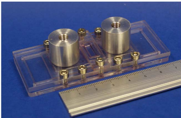
Figure 2. Photograph of the assembled modular culture device with the re-sealable lid attached. doi:10.1371/journal.pone.0052246.g002
