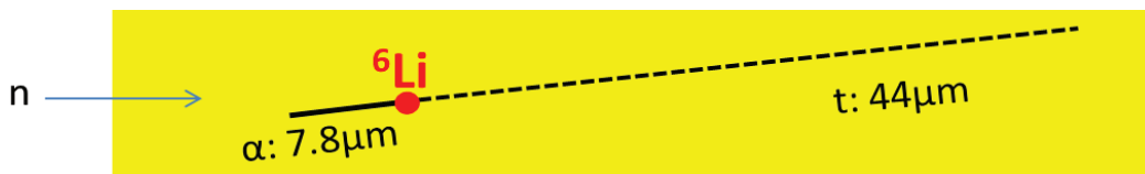
Fig. 1. After the absorption of neutron by {}^6\text{Li} incorporated in a nuclear emulsion of silver halide crystals dispersed in gelatin, an alpha particle and a triton are emitted. A back-to-back topology is formed by their tracks. The expected length of tracks of the alpha particle and the triton are 7.8 \mu\text{m} and 44 \mu\text{m} respectively. These expected lengths were calculated using SRIM.
