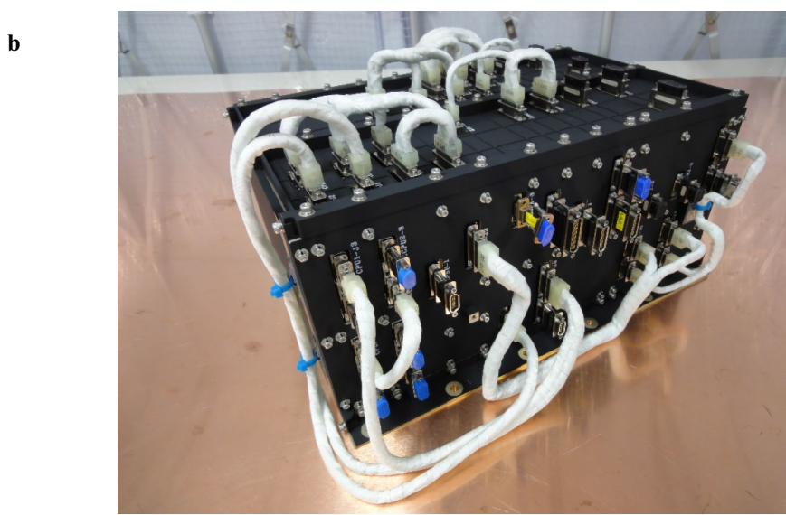
Fig. 2 a Block diagram of the PWE system and b the main electronics box (PWE-E)
